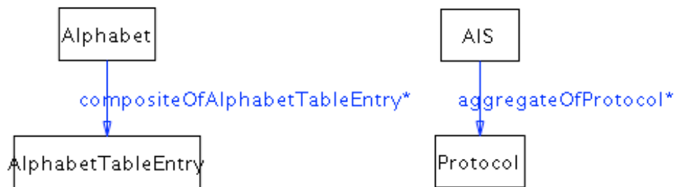
Figure 2 Naming Schemes for Aggregation and Composition
