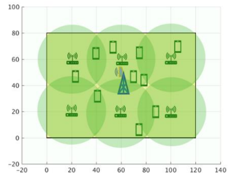
(B) Indoor RLAN devices in the same building as the rooftop FS receiver
