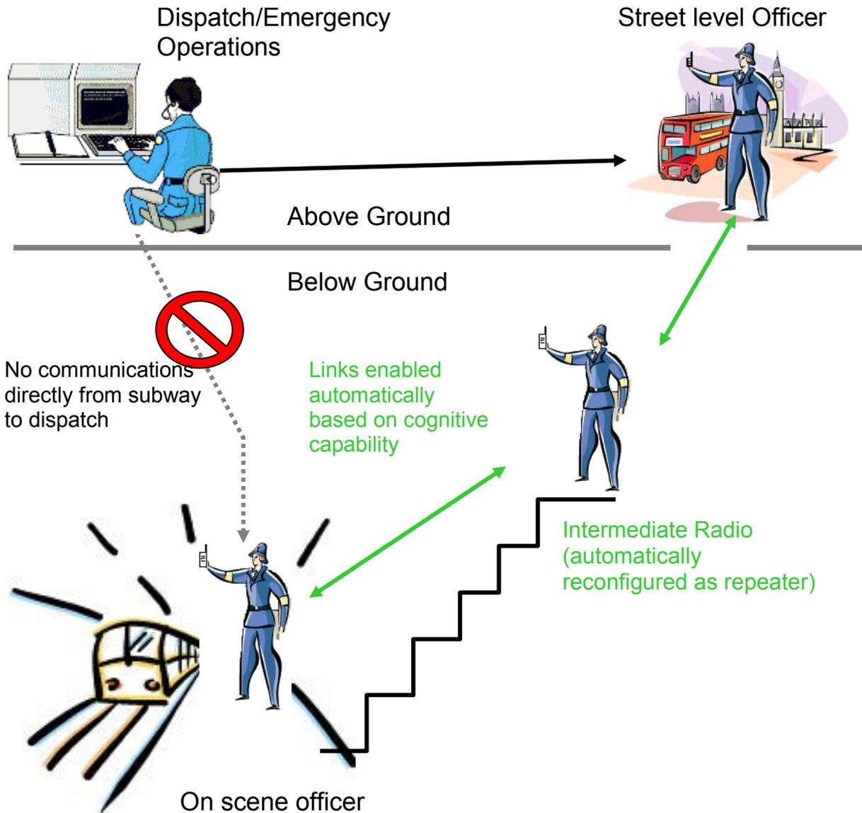
**Figure B-1. Network Coverage Extension Use Case Example**
