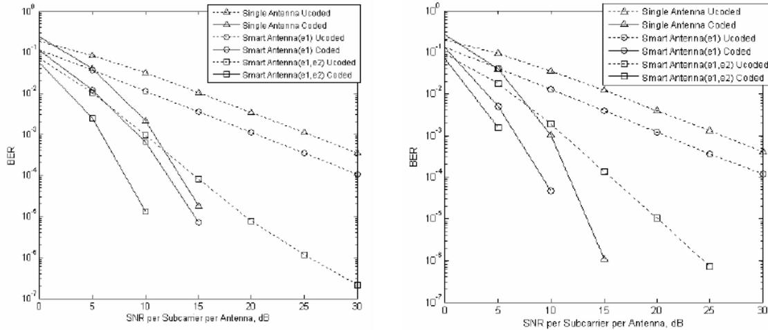
Looks like they screwed up their comparison to the single antenna (as “SNR per Antenna” implies a 3 dB gain going from 1-2 antennas so it is not the traditional apples-to-apples comparison for a given input SNR). However, this is not relevant to the 1 eigenvector versus 2 eigenvectors approach for the same number of antennas.
