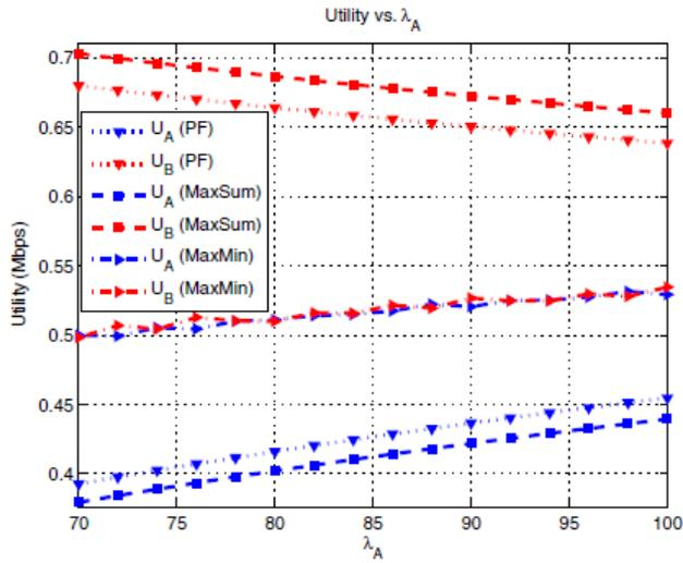
Fig. 5: Each unlicensed user's throughput (Mbps) vs.  $\lambda_A$ .
