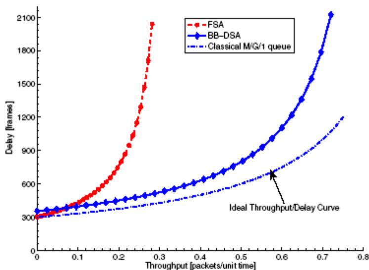
Fig. 4. Delay-throughput results for cell size  $R_{cell} = 1$  km.
