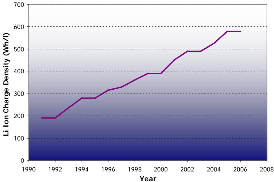
**Figure 33: Improvement Trend for Li Ion Battery Technology<sup>14</sup>**
