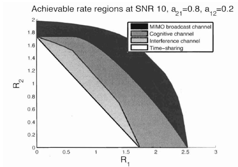
**Figure 17.4 Capacity region of the Gaussian 2x1 MIMO two receiver broadcast channel (outer), cognitive channel (middle), achievable region of the interference channel (second smallest) and time-sharing (innermost) region for Gaussian noise powers  $N_1=N_2=1$ , power constraints  $P_1=P_2=10$  at the two transmitters, and channel parameters  $a_{12}=0.8$ ,  $a_{21}=0.2$ .**
