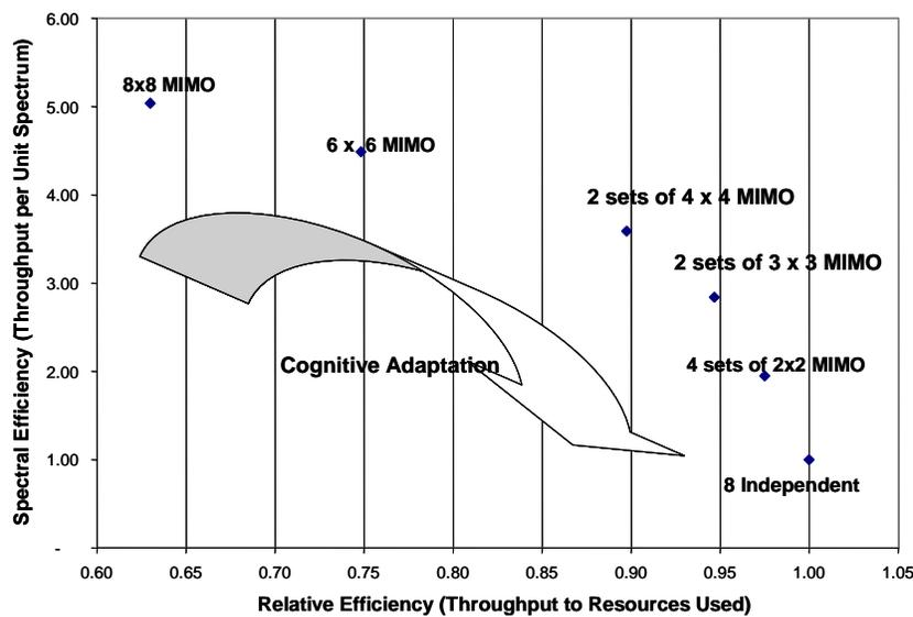
Figure 5.5 Adaptive trades from MIMO and spectrum usage
