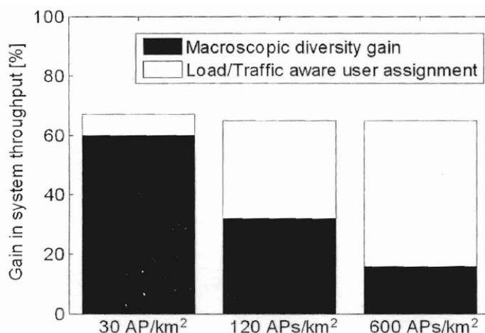
**Figure 30: Gain in asymptotic system throughput for a geographically limited traffic Hotspot where two WLAN (IEEE 802.11a) networks cooperate. As the combined system is noise limited, additional gains can be realized by load aware user assignment. From [Hultell\_07].**
