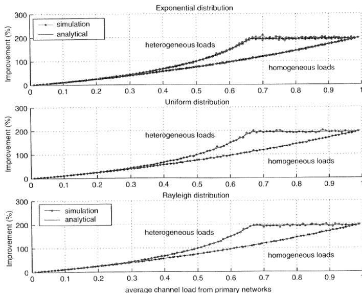
**Figure 7.7 Improvement of spectral utilization for spectral-agile networks: different ON/OFF distributions.**
