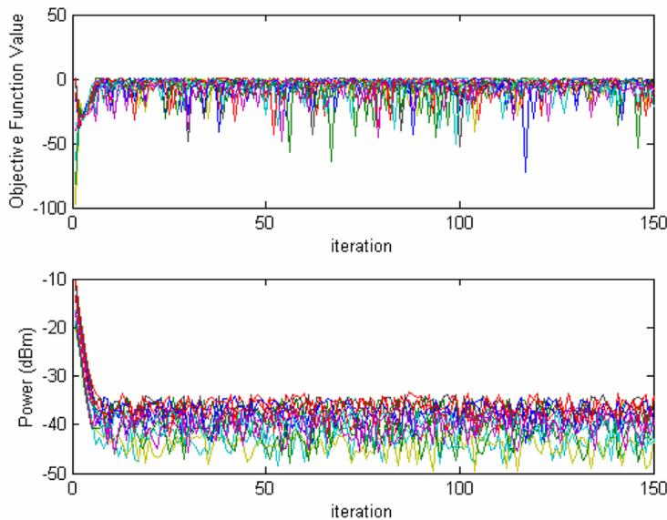
**Figure 15-26** Simulation of an ad hoc network of cognitive radios with synchronous adaptations, utility functions given by eqn. 15-30, and stochastic channel models. The top graph plots the value of each radio’s utility function versus the iteration; the lower plot shows the power levels for each radio versus iteration.
