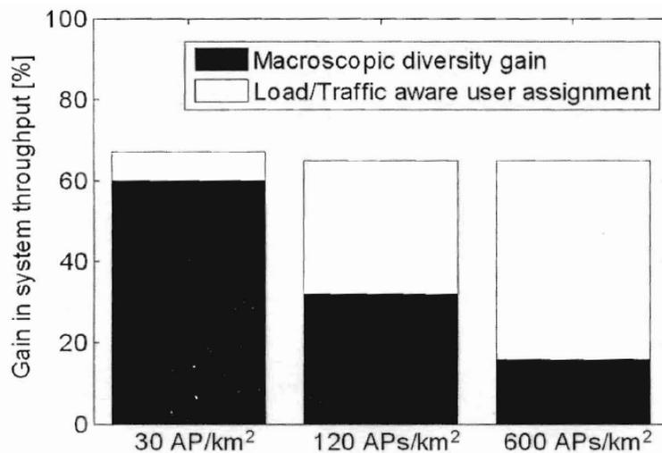
**Figure 6.3** Gain in asymptotic system throughput for a geographically limited traffic hot spot where two WLAN (IEEE 802.11a) networks cooperate. As the combined system is noise limited, additional gains can be realized by load aware user assignment.
