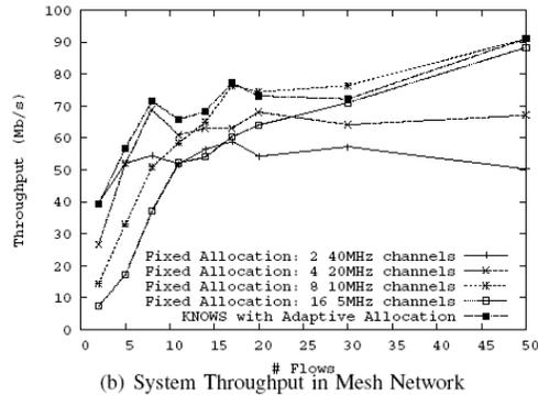
(b) System Throughput in Mesh Network
