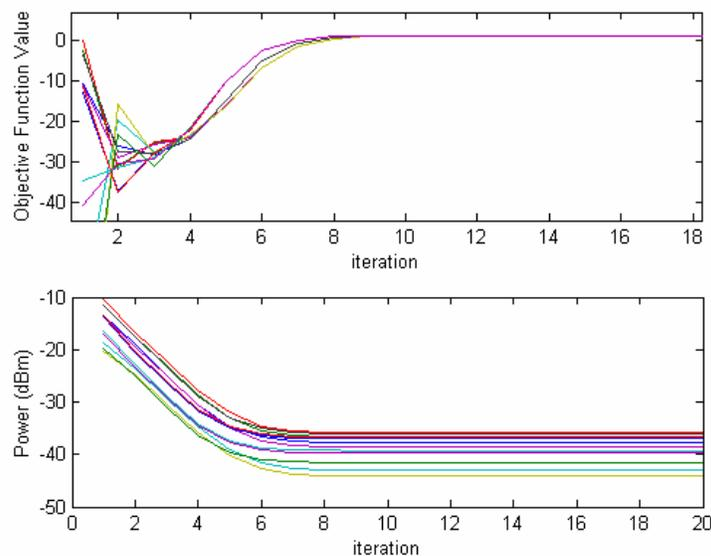
**Figure 22: Deterministic simulation of an ad-hoc network of cognitive radios with synchronous adaptations and utility functions given by eqn. 15-30. The top graph plots the value of each radio's utility function versus the iteration; the lower plot shows the power levels for each radio versus iteration. From Figure 15-25 in [Neel\_06]**
