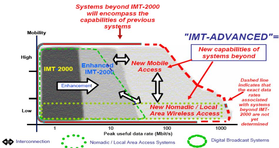
**Figure 32: Representation of data rate and mobility requirements for 4G (IMT-Advanced) systems. From 3G Americas, “Defining 4G: Understanding the ITU Process for the Next Generation of Wireless Technology,” July 2007 Available online: [http://3gamericas.com/PDFs/3G\\_Americas\\_Defining\\_4G\\_WP\\_July2007.pdf](http://3gamericas.com/PDFs/3G_Americas_Defining_4G_WP_July2007.pdf)**
