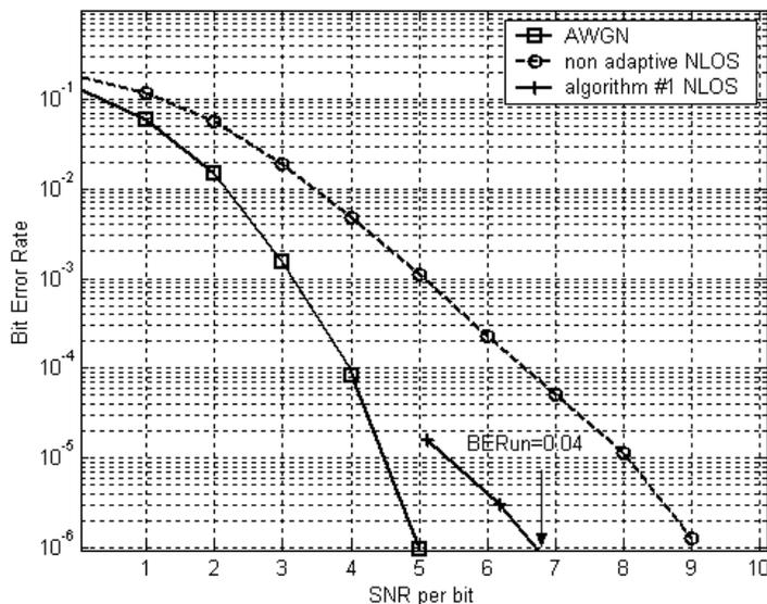
“An average 2dB additional gain is achieved by using the second algorithm versus the first one.”
