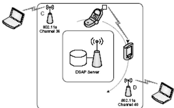
Nodes *A* and *B* are engaged in a UDP transfer on 802.11a channel 40. They continuously move around a square corridor at the rate of 0.75 m/s, always staying about six feet from each other. Nodes *C* and *D* sit at the opposite corners of the corridor and send UDP data to their neighbors on (non-overlapping) channels 36 and 40, respectively. *C* and *D* operate with reduced power (0 dBm) and only interfere in areas of their line-of-sight (LOS).
