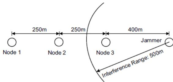
Fig. 9. Network setup for the unicast simulations.
