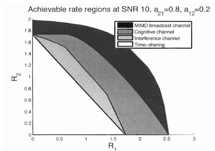
**Figure 15: Capacity region of the Gaussian 2x1 MIMO two receiver broadcast channel (outer), cognitive channel (middle), achievable region of the interference channel (second smallest) and time-sharing (innermost) region for Gaussian noise powers  $N_1=N_2=1$ , power constraints  $P_1=P_2=10$  at the two transmitters, and channel parameters  $a_{12}=0.8, a_{21}=0.2$ . From Figure 17.4 in [Devroye\_07].**
