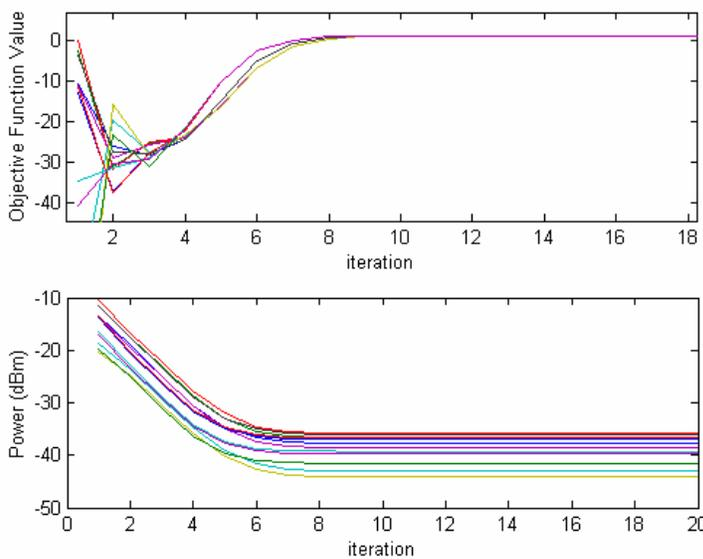
**Figure 15-25 Deterministic simulation of an ad-hoc network of cognitive radios with synchronous adaptations and utility functions given by eqn. 15-30. The top graph plots the value of each radio's utility function versus the iteration; the lower plot shows the power levels for each radio versus iteration.**
