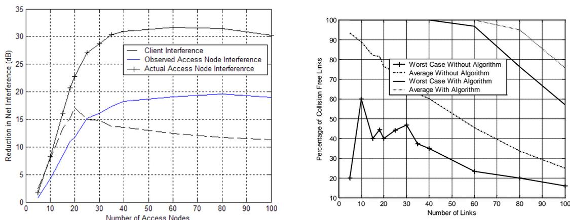
**Figure 26: By ensuring all observations in the network satisfy the BSI condition, significant reductions in interference were achieved for coexisting WLANs in infrastructure mode (left) and in collision probabilities in ad hoc mode (right). From Figures 6 and 8 in [Neel\_07].**
