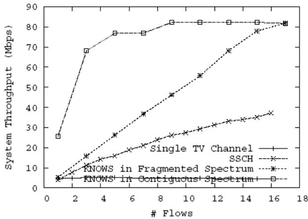
Fig. 10. System Throughput with Disjoint UDP Flows
