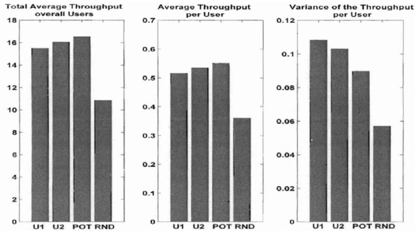
**Figure 18: Total Average Throughput, Average Throughput per user and Variance Throughput per user (U1 = selfish users with minimum regret learning algorithm implementation; U2 = cooperative users with minimum regret learning algorithm implementation; POT = cooperative users with potential game implementation; RND = equal probability random channel allocation). From Figure 28.6 in [Comanciu\_07].**
