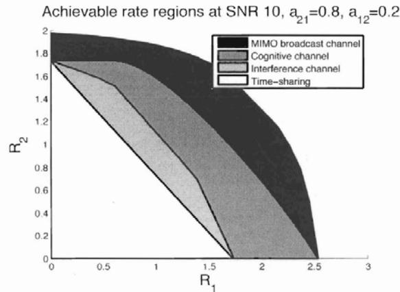
**Figure 8: Capacity region of the Gaussian 2x1 MIMO two receiver broadcast channel (outer), cognitive channel (middle), achievable region of the interference channel (second smallest) and time-sharing (innermost) region for Gaussian noise powers  $N_1=N_2=1$ , power constraints  $P_1=P_2=10$  at the two transmitters, and channel parameters  $a_{12}=0.8$ ,  $a_{21}=0.2$ . From Figure 17.4 in [Devroye\_07]**
