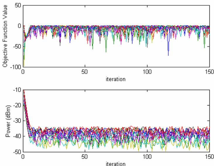
**Figure 23: Simulation of an ad hoc network of cognitive radios with synchronous adaptations. The top graph plots the value of each radio’s utility function versus the iteration; the lower plot shows the power levels for each radio versus iteration. From Figure 15-26 in [Neel\_06]**
