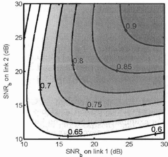
**Figure 16: CSR availability when both links satisfy Condition I. SNR<sub>b</sub> denotes the mean SNR per branch. From Figure 23.7 in [Lu\_07]**
