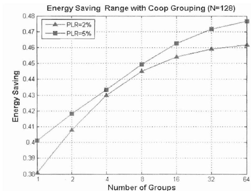
**Figure 17: A cooperative retransmission scheme was reported to save energy in a WLAN system as a function of the Packet Loss Ratio (PLR) and the number of groups with a fixed number of nodes (128). However, diminishing returns on groupings is seen. From Figure 25.8 in [Zhang\_07]**
