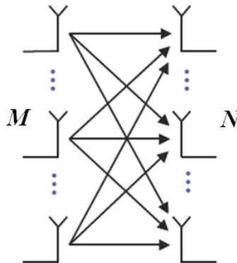
**Figure 13: In a MIMO system, there are multiple antennas at the transmitter and multiple antennas at the receiver. If there are  $M$  transmit antennas and  $N$  receive antennas, there are  $M \times N$  propagation paths between the antennas in the system.**
