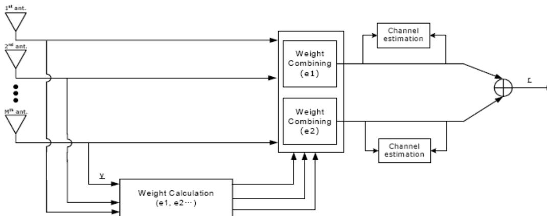
MRC combining formed from two channel estimates ( $\hat{h}$ ), two eigenvectors ( $\underline{e}$ ) and input samples ( $\underline{y}$ ).
