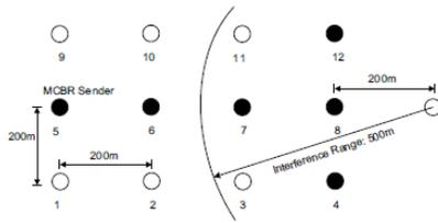
Fig. 12. Network setup for the MCBR multicast application, where solid black circles represent the nodes in the multicast group.
