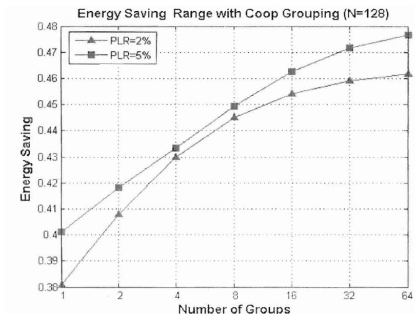
**Figure 17: A cooperative retransmission scheme was reported to save energy in a WLAN system as a function of the Packet Loss Ratio (PLR) and the number of groups with a fixed number of nodes (128). However, diminishing returns on groupings is seen. From Figure 25.8 in [Zhang\_07]**
