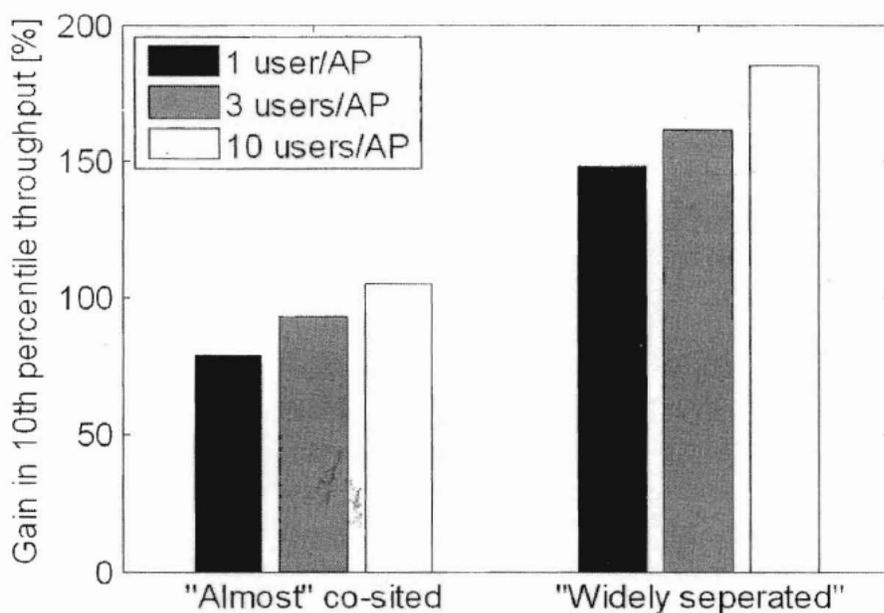
**Figure 6.2: Gain in asymptotic user throughput for the 10<sup>th</sup> percentile (“coverage”) for uplink transmission in a case where three operators cooperate.**
