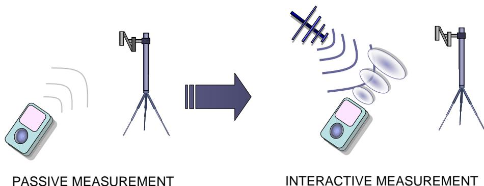
**Figure 46: Because CRs are expected to respond to and interact with a more complex ecosystem and exhibit a greater range of responses than traditional radios would, interactive measurements will need to be more extensive to ensure proper operation of cognitive radios.**
