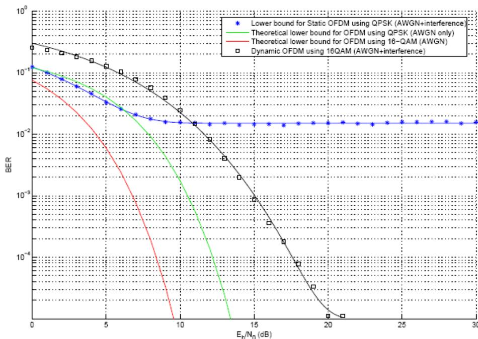
[I’m nearly certain that the AWGN BER curves in Fig 5 are mislabeled. The red line is actually QPSK (labeled as 16-QAM) and the green line is 16-QAM (labeled as QPSK).]
