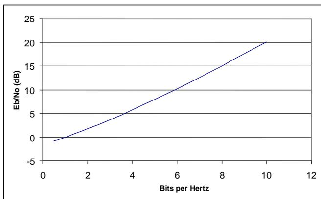
Figure 5.2: Shannon EB [energy per bit] for various spectral efficiency values.
