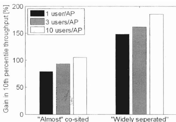
**Figure 31: Gain in asymptotic user throughput for the 10<sup>th</sup> percentile (“coverage”) for uplink transmission in a case where three operators cooperate. From [Hutell\_07]**
