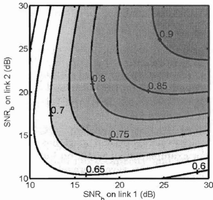
Figure 23.7 CSR availability when both links satisfy Condition I. SNR<sub>b</sub> denotes the mean SNR per branch.
