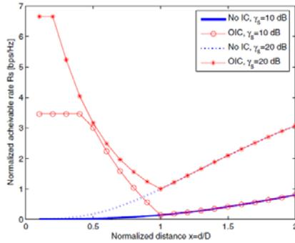
Fig. 5. Normalized achievable rate as a function of the normalized distance of the secondary RX from the primary BS. “No IC” is without Interference Cancellation. Here  $\beta_p = 20$  [dB], propagation coefficient is  $\nu = 3$ .
