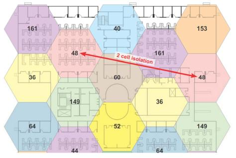
Wi-Fi uses combination of Energy Detect (ED) and/or Preamble Detect (PD) with <u>Reuse={3-25}</u> networks <u>using C/N operation</u> and consumer grade components
