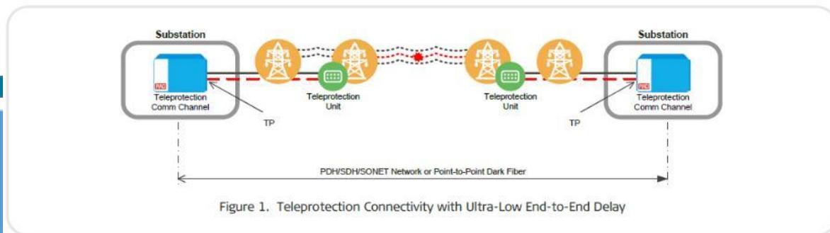
Figure 1. Teleprotection Connectivity with Ultra-Low End-to-End Delay
