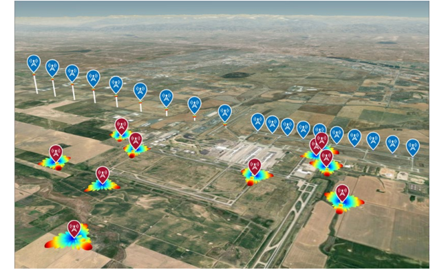
Simulated RADALT flight path with 5G antenna models
