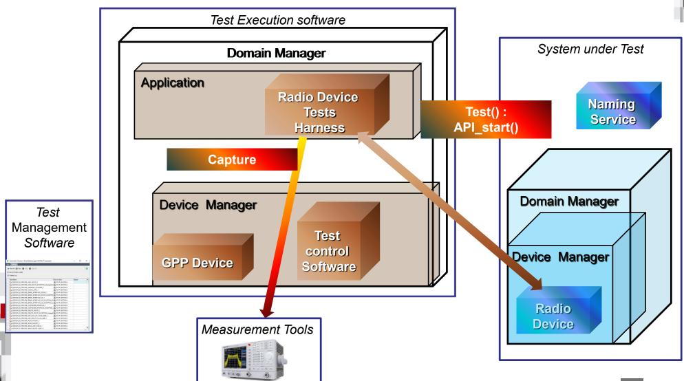
Example of Radio Device API Platform testing
