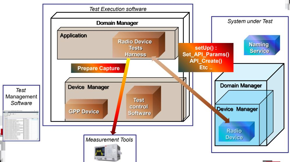
Example of Radio Device API Platform testing
