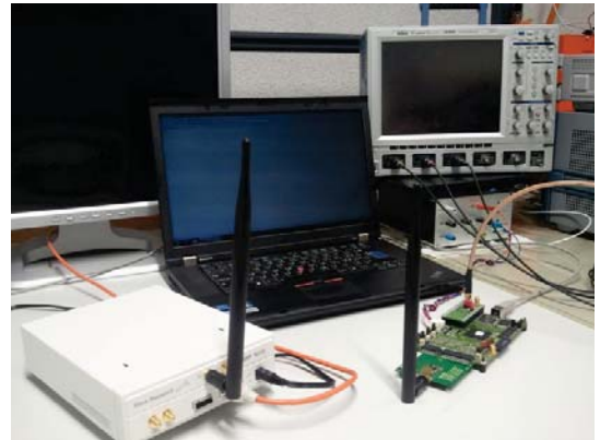
Fig. 7. Testbed setup with USRP N200 and receiver board.
