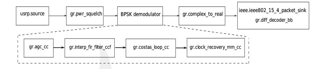
A new block ieee.ieee802\_15\_4\_packet\_sink coombined with gr.diff\_decoder\_bb is add to GNU Radio.
