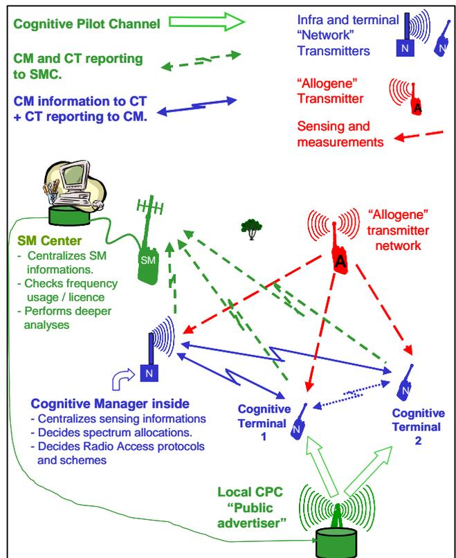
Figure 9: Illustration of a possible network structure for sensing + spectrum monitoring by using cognitive radios.
