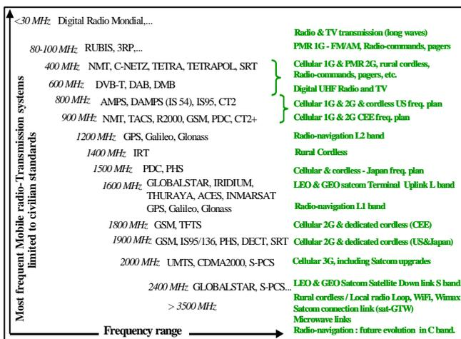
Figure 1: Civilian communication signals to be processed by SM
