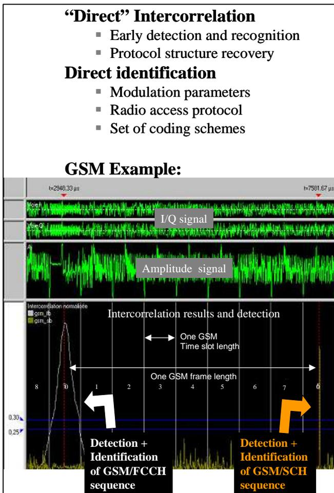
Figure 6 : Examples of data aided processing of radio-communication signals (GSM, UMTS, DVB-T & LTE)
