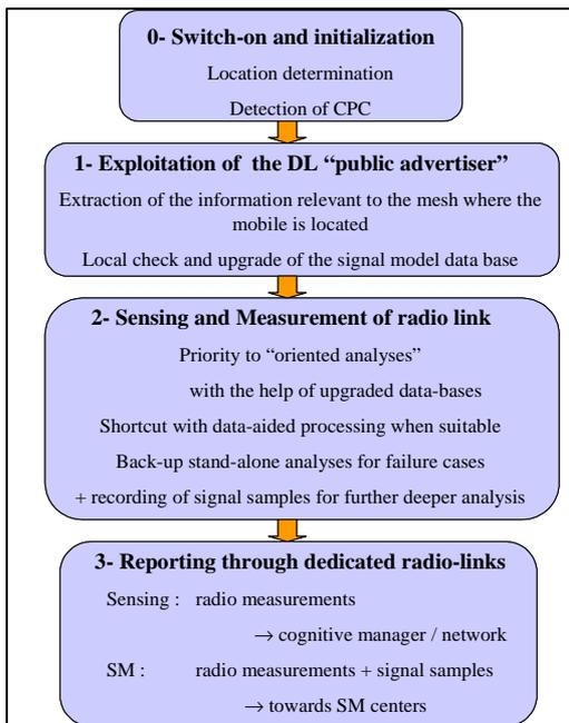
Figure 8 : Example of sensing + measurement protocol for a cognitive terminal (extended from [12]).
