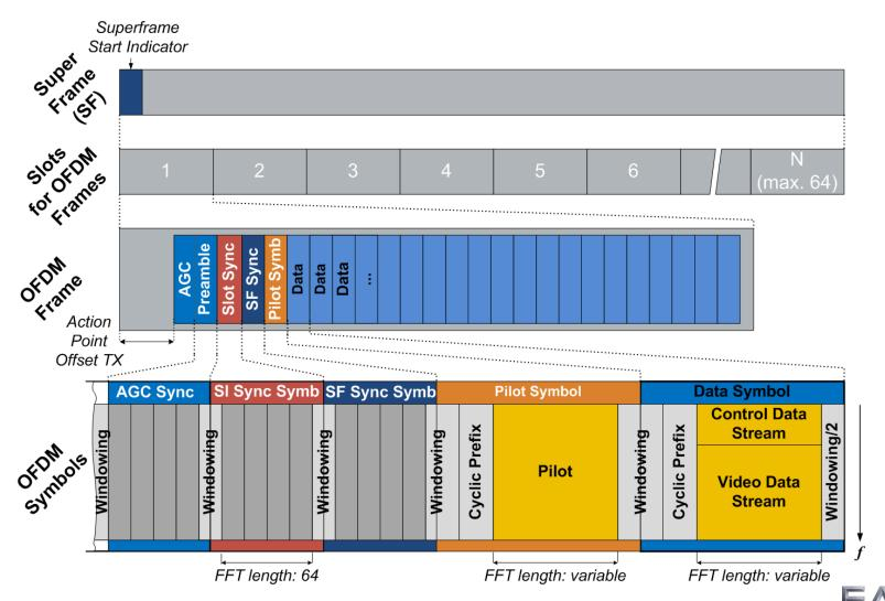
For Channel access of different users (UGV, UAV, base station)
