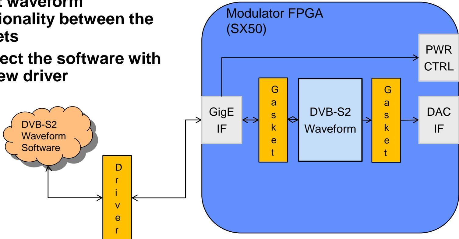
**The modulator core VHDL was not modified to support the BDR-1 platform. All new code was limited to the gaskets.**
