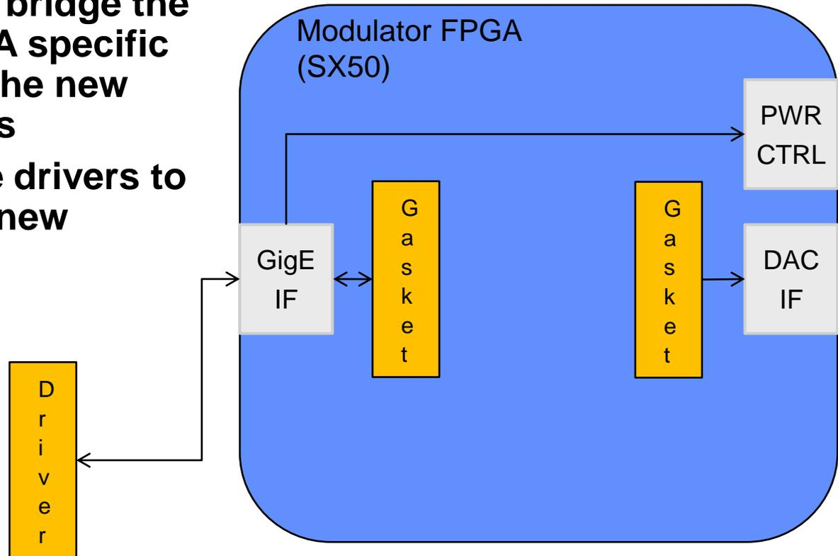
**Gaskets reduce configuration management issues by not changing the platform specific and or waveform specific features during a porting effort.**
