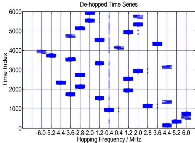
Figure 7. De-hopped Signal Time Series Plotted at All Output Ports of De-hopping Channelizer
