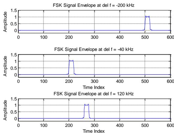
Figure 9. 8-FSK Demodulation Channelizer Output for 1.2 MHz Hopping Center
