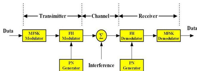
Figure 1. High level view of MFSK/FH system
