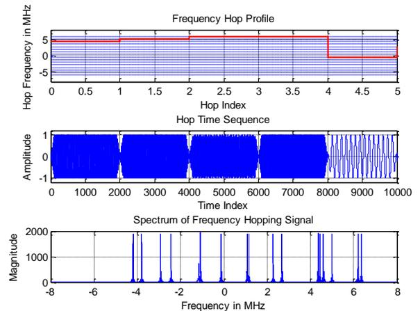
Figure 6. Frequency Hopping Profile and Hop Time Series
