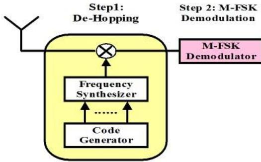
Figure 3. Conventional FH demodulator
