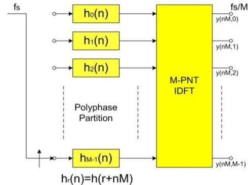
Figure 2. Standard  $M$ -path Polyphase Down Converting Channelizer
