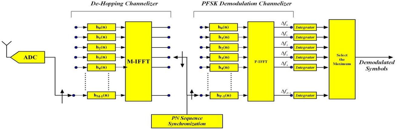
Figure 5. Proposed full digital FHSS demodulator
