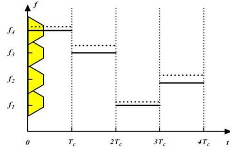
Figure 4.  $M$ -path Channelizer Aliases Hopping Frequencies onto Baseband
