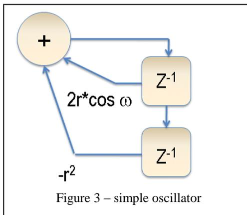
Figure 3 – simple oscillator
