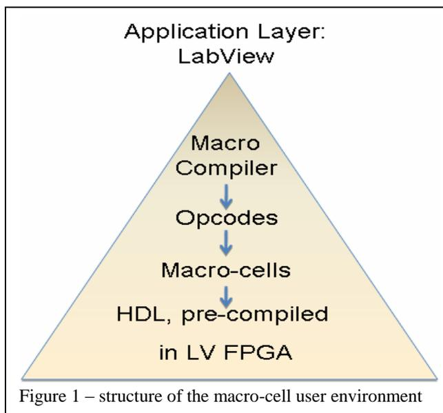
Figure 1 – structure of the macro-cell user environment
