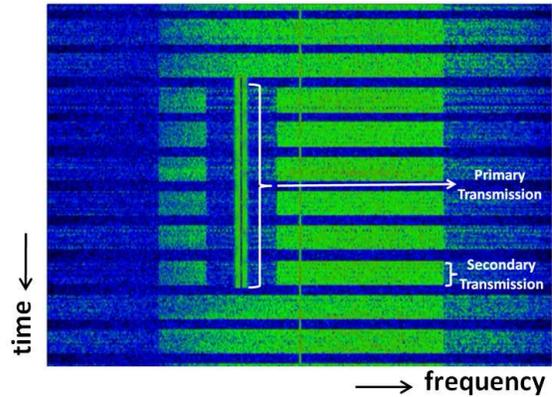
Fig. 2. Spectrogram illustrating the DSA operation
