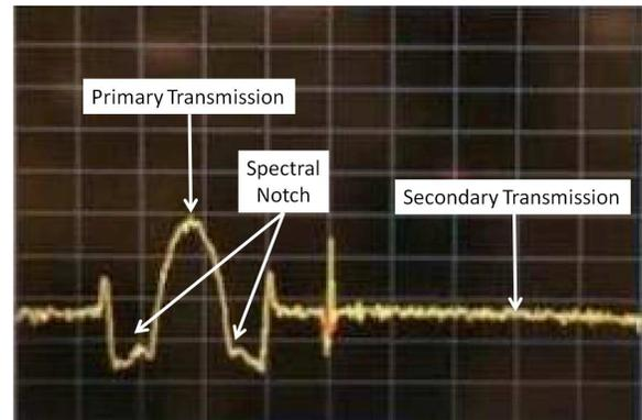
Fig. 6. Spectrum showing the co-existence of primary and secondary systems. [x-axis: 200 kHz/div, y-axis: 10 dBm/div]
