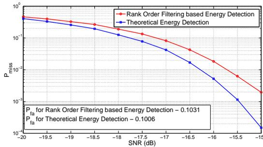
Fig. 4. Performance of the ROF based sensing algorithm
