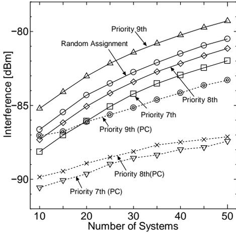
Fig.9 The given interference performance toward low priority channels while the average number of channel aggregation is 10.
