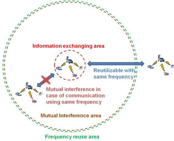
Fig1. Three areas for frequency assignment.
