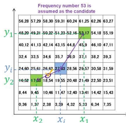
Fig.5 Frequency decision example with 2<sup>nd</sup> priority at the location with 1<sup>st</sup> priority frequency number as 27.
