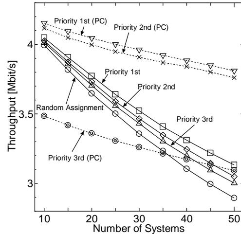
Fig.12 The throughput performance toward high priority channels while the average number of channel aggregation is 10.
