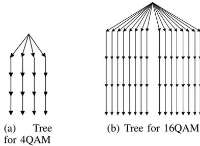
Fig. 2. Detection Tree for FSD
