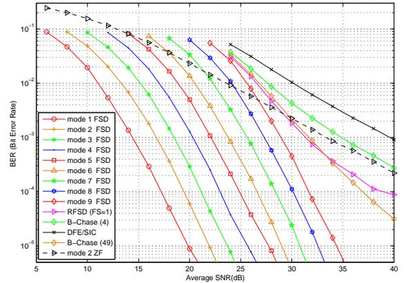
Fig. 7. BER performance of FSD over Adaptive Modulated MIMO  $4 \times 4$
