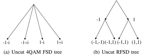
Fig. 3. 4QAM FSD/RFSD Processing
