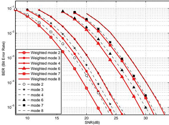
Fig. 6. Variation of BER with SNR of FSD in a  $4 \times 4$  AM-MIMO
