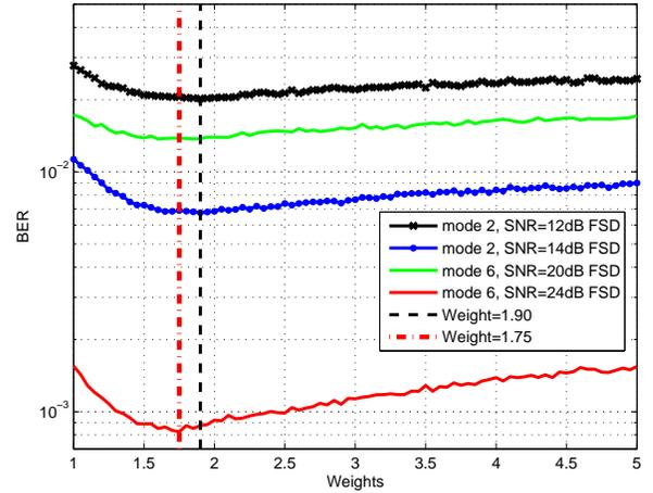
Fig. 4. BER of FSD in a  $4 \times 4$  AM-MIMO with Varying Weights
