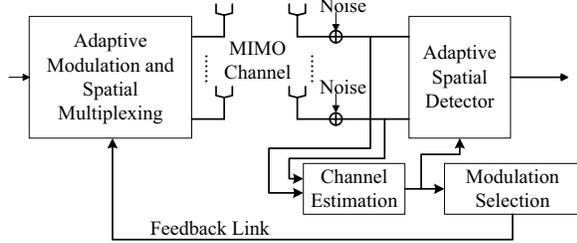
Fig. 1. AM System Architecture For Flat Fading MIMO Channels
