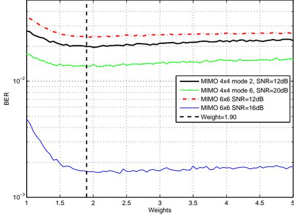
Fig. 5. BER of RFSD in an AM-MIMO System with Varying Weights
