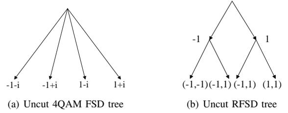
Fig. 3. 4QAM FSD/RFSD Processing
