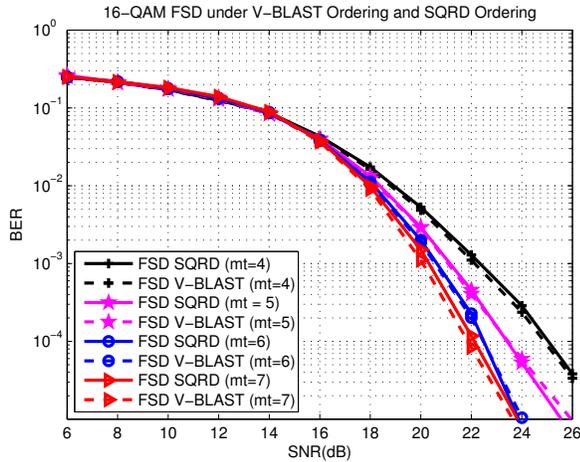
**Fig. 4.** SQRD/V-BLAST FSD BER Performance Comparison
