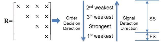
Fig. 3. Order Decision and Signal Detection Direction by SQRD Preprocessing
