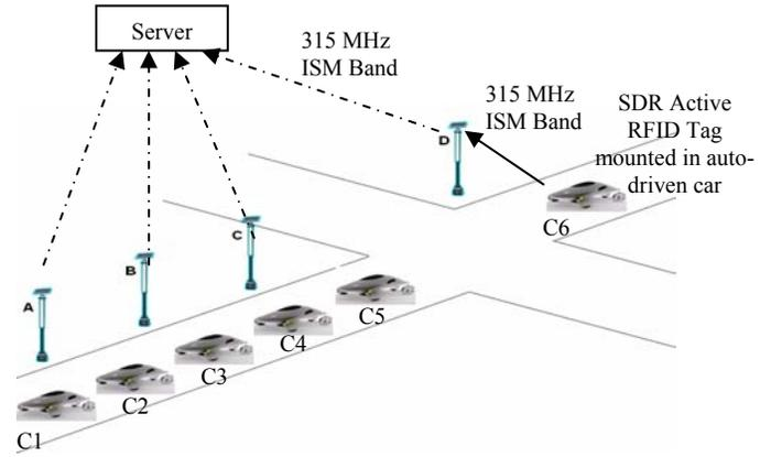
Figure 4. Block diagram of the car location detection network with multiple RFID reader system
