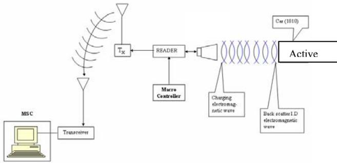
Figure 3. Block diagram of the car location detection with single RFID reader system
