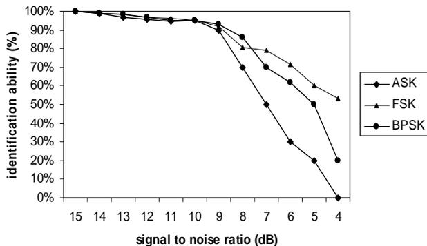
Figure 8. Percentage of correct identification performance for ASK, FSK and BPSK modulated signal using WT
