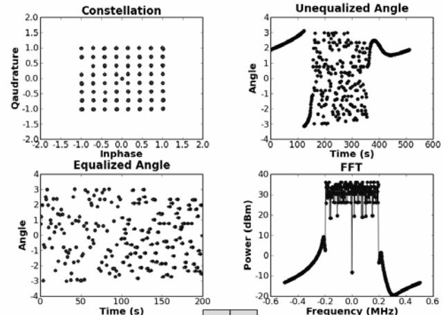
Figure 7. Results of using QAM64 subcarrier modulation.
