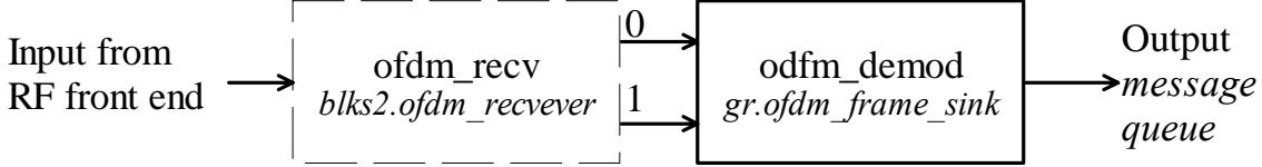
**Figure 3. GNU Radio OFDM demodulator block diagram (blk2impl/ofdm.py:ofdm\_demod). The ofdm\_receiver block is a hierarchical block in Python and is shown in Figure 3.**
