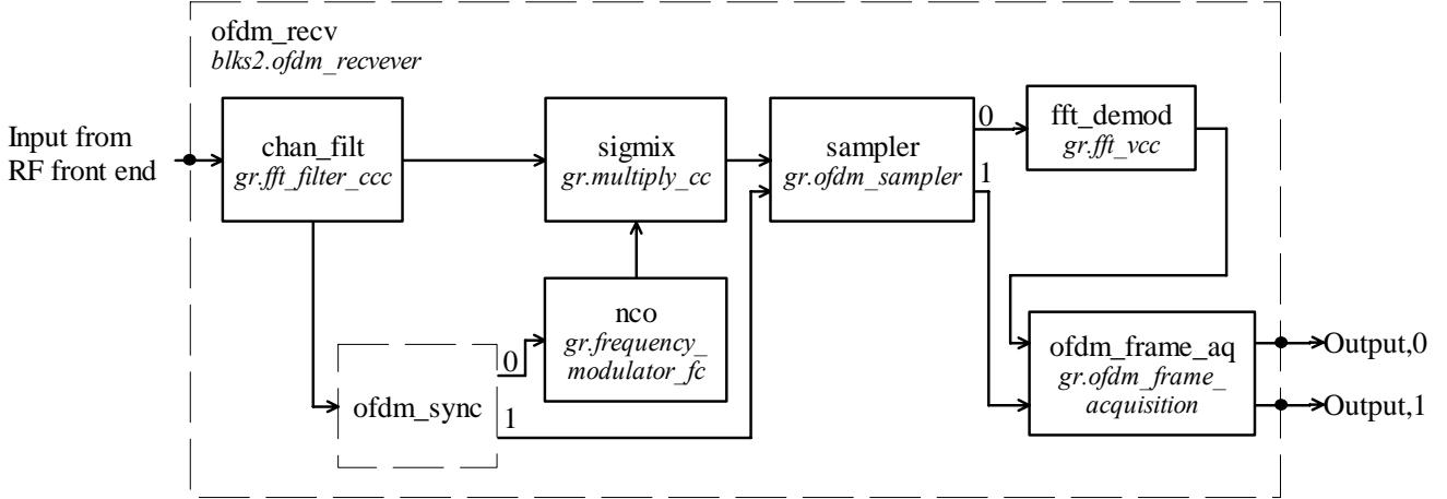
**Figure 2. GNU Radio OFDM receiver (blk2impl/ofdm\_receiver.py:ofdm\_receiver). The ofdm\_sync block is a hierarchical block in Python that can be replaced for different timing and frequency acquisition functions and techniques (see Section 4).**
