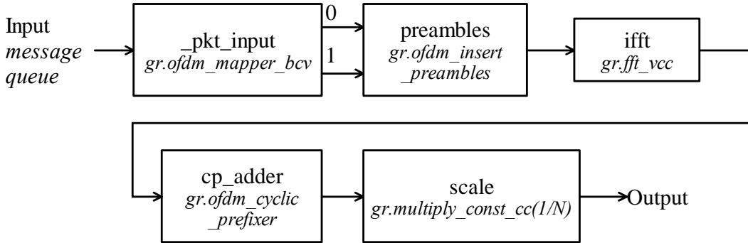
**Figure 1. GNU Radio OFDM modulator block diagram (blk2impl/ofdm.py:ofdm\_mod).**
