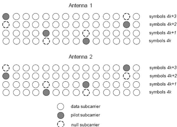
Figure 1 A cluster structure for MIMO system using two transmit antennas
