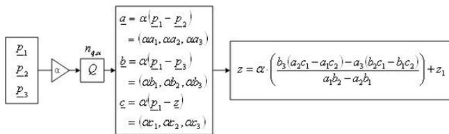
Figure 5 The simple block diagram of fixed-point design for advanced 2D interpolation algorithm
