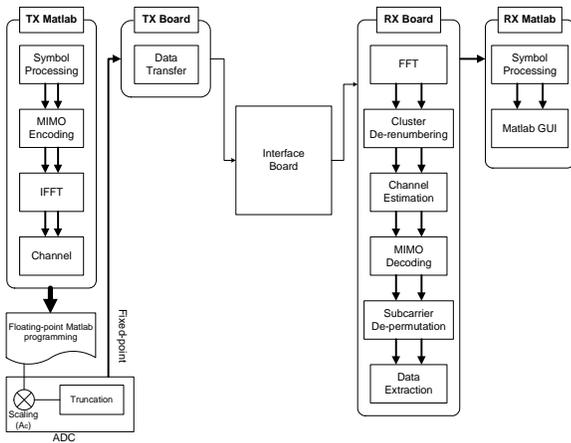
Figure 4 the block diagram for implementation of advanced 2D interpolation technique
