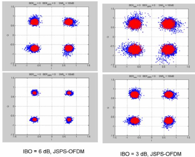
Figure 9: Receiver constellations, top: no PD or PAPR reduction, bottom: combined PD and PAPR reduction.
