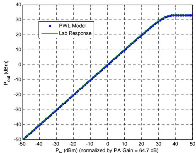
Figure 3: Lab Response and Piece-wise Linear Model
