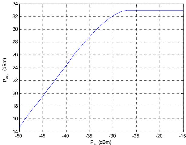
Figure 2: Lab Measurement of a state of the art PA
