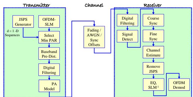
Figure 1: JSPS-OFDM System Model
