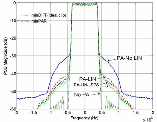
Figure 7: Transmit spectrum for 9 dB IBO.
