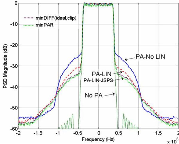
Figure 8: Transmit spectrum for 6 dB IBO.
