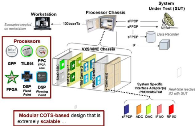
Figure 1 Diagram of RES components and Radar Under Test.
