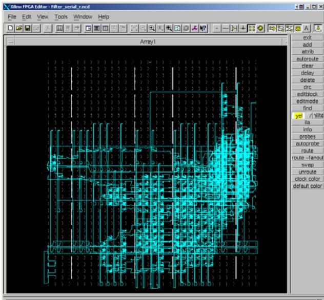
Figure 3 FPGA layout of digital filter generated using HDL Coder.
