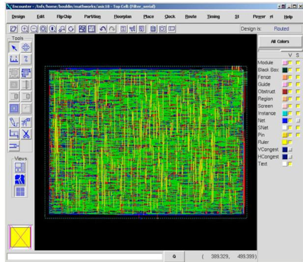
Figure 4 ASIC layout of digital filter generated using HDL Coder for TSMC 180 nm process.
