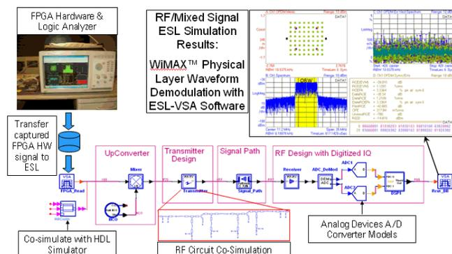
Figure2 - Integrated RF/Mixed Signal ESL system simulation with HDL and RF circuit co-simulation, and VSA software.
