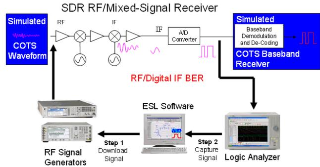
Figure 5 - Using ESL COTS waveform sources and receivers to test SDR RF/mixed-signal receiver hardware.
