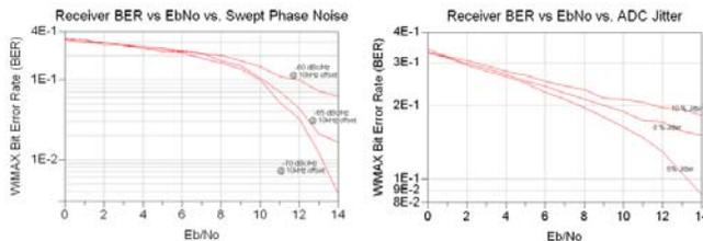
Figure 4 - SDR RF Receiver Simulation Results- BER versus Phase Noise (left) and BER versus ADC Jitter (right)..
