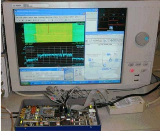
Figure 6 - “RF-Aware” FPGA test setup using RF ESL simulation inside the logic analyzer.
