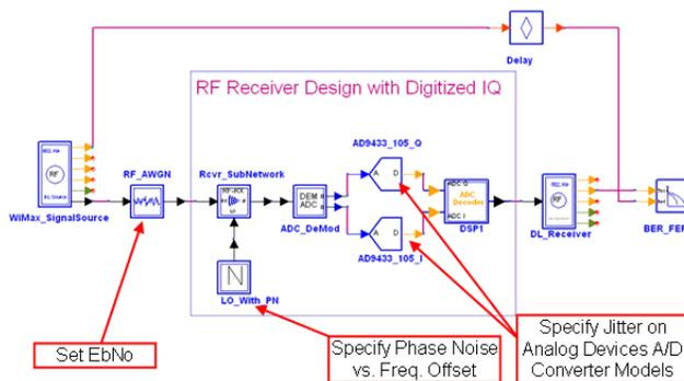
Figure 3 - WiMAX™ COTS waveform for SDR RF receiver design.
