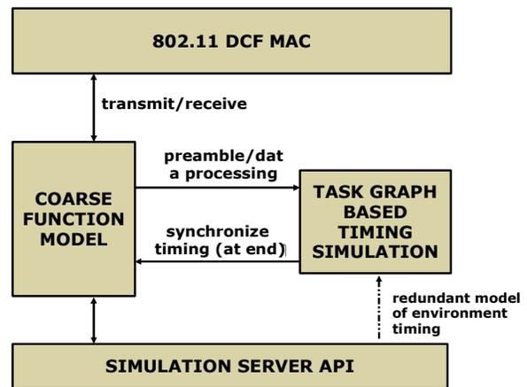
Fig. 8: Layout of a generic platform architecture simulated with the system simulation server and reusing the 802.11 DCF MAC software layer
