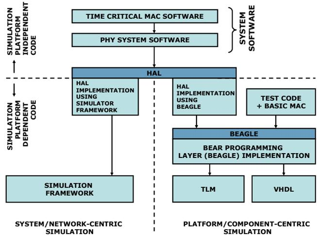
Fig. 3: System software layers (ARM processor) and their relation with the different simulation levels.
