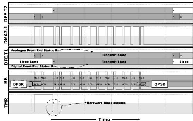
Fig. 6: Simulation results for the transmission of a data packet in MIMO mode.
