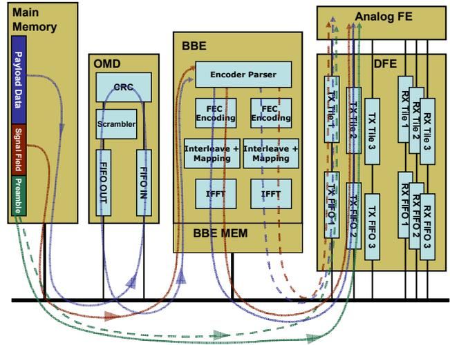
Fig. 5: The data path through the main platform components for the transmission of an 802.11n data packet.
