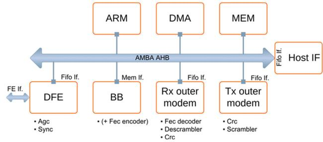
Fig. 2: IMEC SDR digital baseband platform
