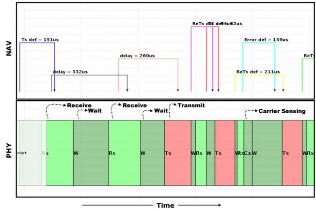
Fig. 7: Simulation results for a DCF 802.11 MAC terminal
