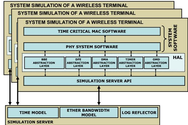
**Fig. 4: Simulating several terminals using calls to the system simulation servers API**
