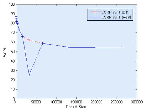
Figure 6 - USRP Component (OSSIE): non-signal processing part CPU load
