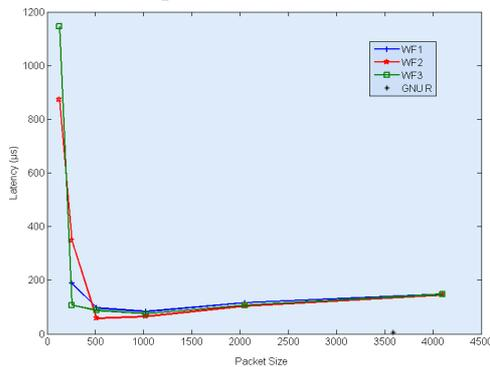
Figure 8 - Inter-component latency (small packet size)
