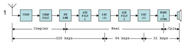
Figure 1 - FM receiver waveform
