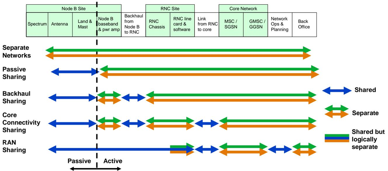
Figure 2. Infrastructure sharing possible with traditional radios. Source: UK Office of Communications (OFCOM).
