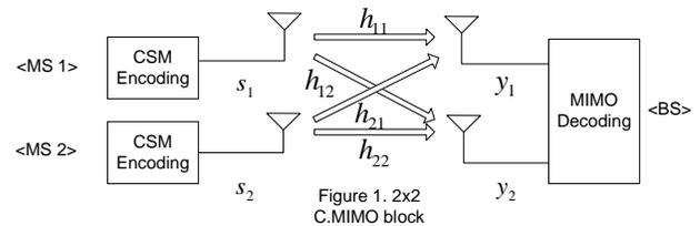
Figure 1 shows example of CSM system consisting of two mobile stations and one base station where each mobile station has single antenna and base station has two antennas. Each mobile station can transmit independent data on the same time and the same frequency. At the base station, received signal vector can be expressed as below.
