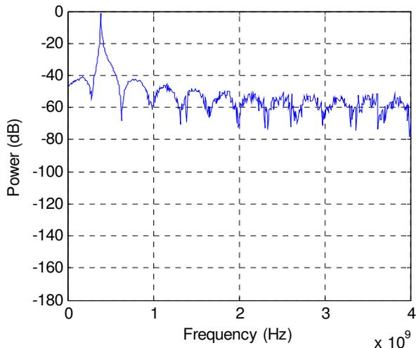
Figure 5: Power spectral density (PSD) of output of time-interleaved ADC with pseudo-random jitter and skew ( $t_{adc} = 0.1$ ) shows harmonics.
