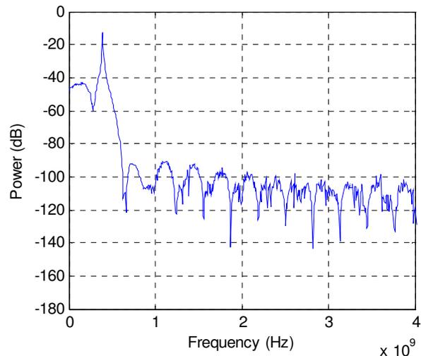
Figure 6: Power spectral density (PSD) of output of interpolator and RRC filter with pseudo-random jitter and skew ( $t_{adc} = 0.1$ ) shows harmonics with significant improvement.
