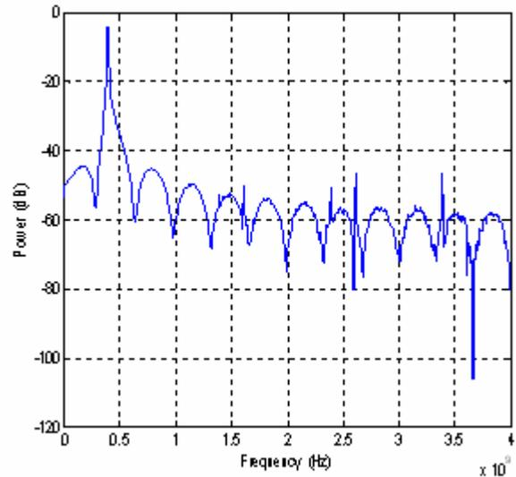
Figure 4: power spectral density (psd) of output of time-interleaved adc with jitter = 0 and skew ( $t_{adc}$ ) = 0.1 shows harmonics
