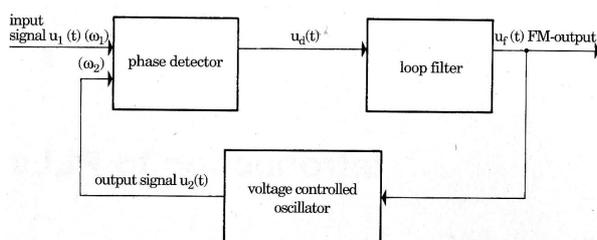
The loop filter is designed such that its DC output level is adjusted proportionately to the phase offset between the input sinusoid and the VCO output sinusoid. Assuming the feedback loop is stable, the input to the VCO will adjust the phase of the output sinusoid until its phase offset matches that of the input sinusoid.
