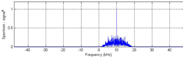
Unfortunately the technique is not as successful at extracting higher order M-QAM based carrier signals. The plots below show the fourth-power signal spectrum for 16-QAM and 64-QAM. The magnitude of the carrier component is shown to diminish relative to the message frequency components as the QAM order increases.
