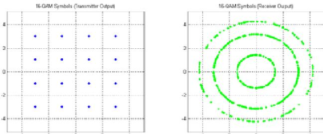
The received symbol constellation is spinning as predicted. And the phase rotation can be defined as:
