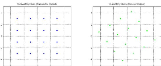
The constellation plots show the receiver QAM symbols are rotated by  $0.2\pi$  radians as predicted. Assuming that  $f_r \neq f_i$  and that  $(f_r - f_i) = 10\text{Hz}$  then the received baseband symbol stream can be defined as:
