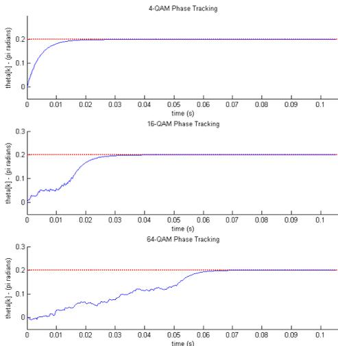
In addition, the plots below show that the algorithm successfully tracks a varying relative carrier phase at the receiver:
