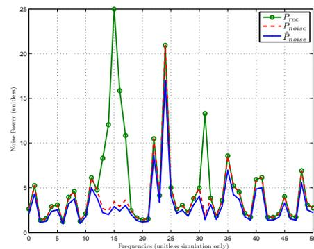
Fig. 2. The received power, the actual noise power at the receiver, and the estimated noise power
