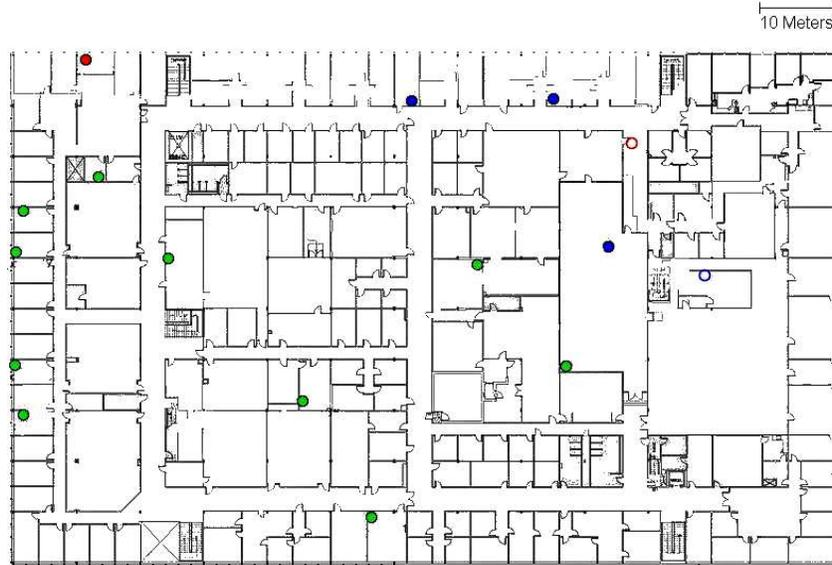
Fig. 1. The placement of the Emulab nodes with USRP devices in the MEB. The green circles represent available nodes. The red circles represent nodes that are out-of-service. The blue circles represent nodes that are in-use. The unfilled circles are the nodes on a different floor than the map.
