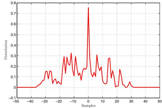
Fig. 5. Normalized correlation of the actual signal power with the average of signal power of the nodes
