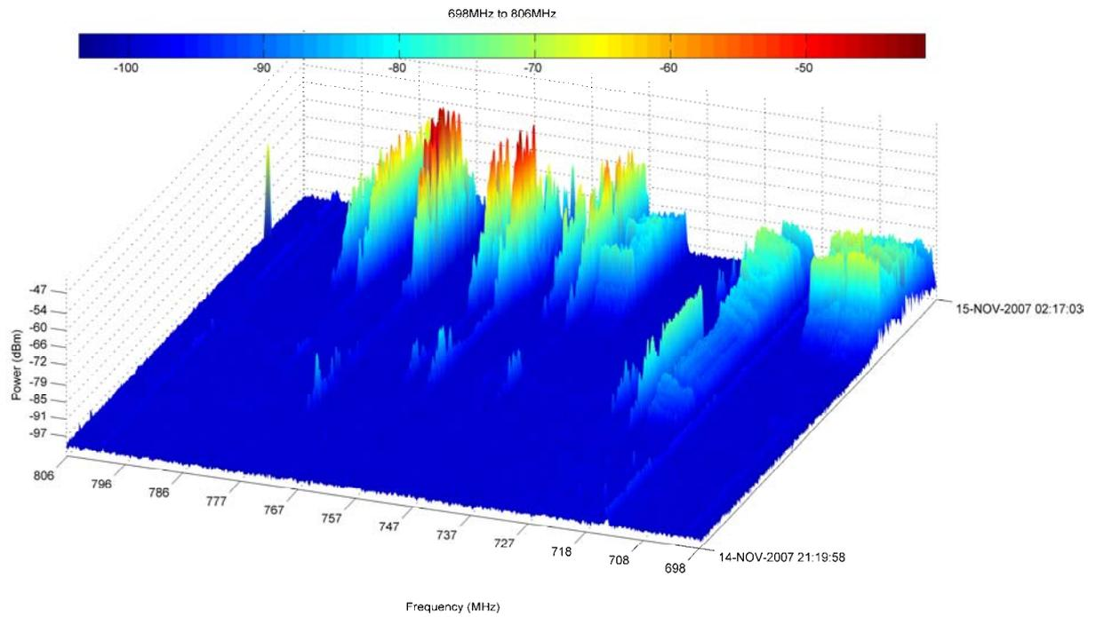
Figure 3. A plot of the spectrum occupancy for the route shown in Figure 2. Frequency is shown on the X-axis, time and date are represented on the Y-axis and the received power levels in dBm are displayed on the Z-axis.
