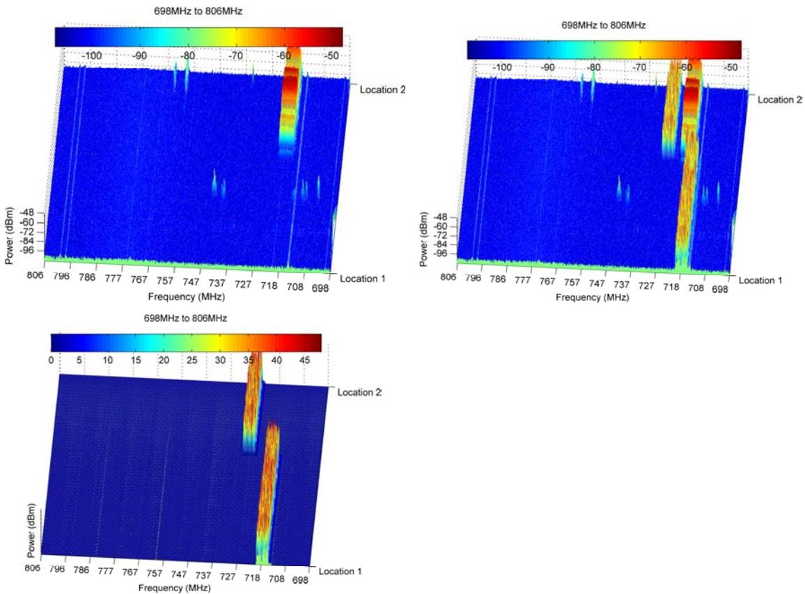
Figure 6,7,8 (clockwise from the top). A plot of spectrum usage in the Topeka, Kansas region. The main visible received signal is a MediaFLO service centered at 719MHz. The plot on the top right is the same spectrum usage plot with the simulated injected OFDM-based dynamic spectrum access secondary user transmission. The plot on the bottom left shows the isolated injected OFDM secondary-user transmission.
