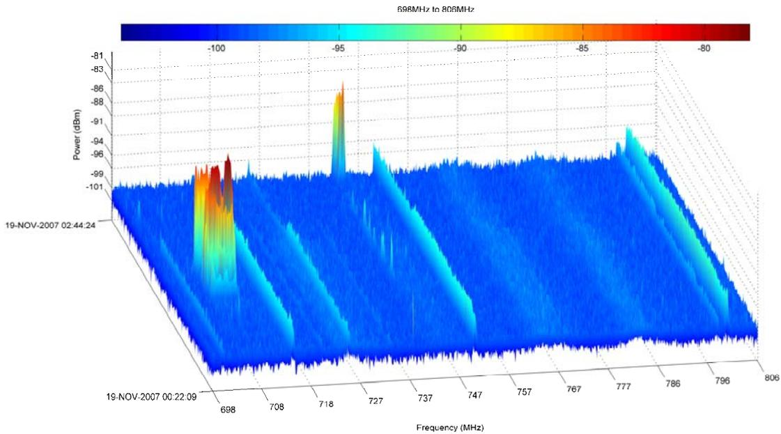
Figure 5. A three-dimensional spectral-occupancy plot for the route shown in Figure 4. Frequency is displayed on the X-axis, time and date information on the Y-axis and received power levels in dBm on the Z-axis.
