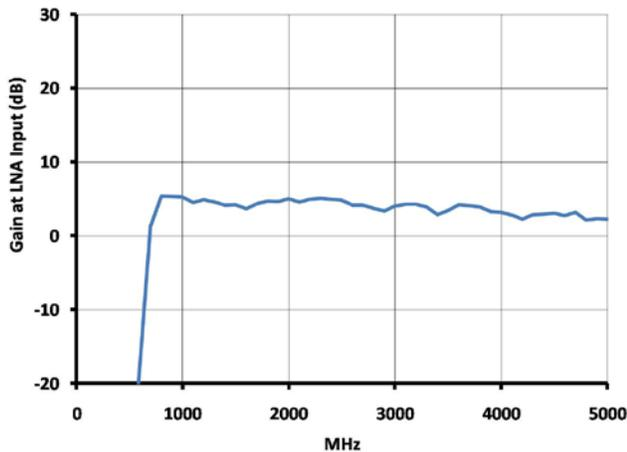
Figure 4: Flatness of Antenna, Cable, and High-Pass Filter
