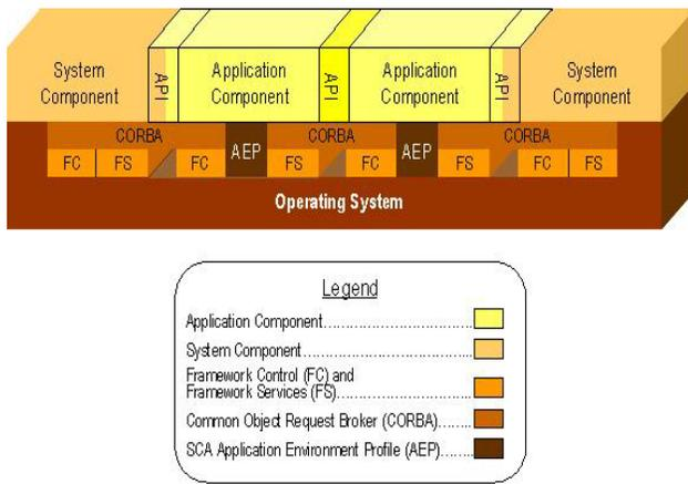
Figure 8. SCA Architecture Layers. (Source: SPAWAR)
