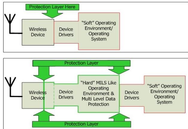
Figure 13. HAWCS™ architecture provides waveform developers with an approach for securing the SDR platform from wireless and network “hacking”.
