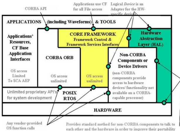
Figure 9. Architecture view showing interaction boundaries between SCA applications, core frameworks, operating systems, device drivers and hardware.
