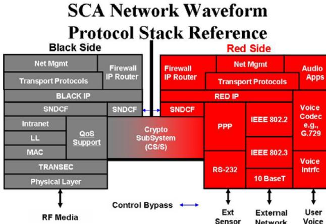
Figure 11. Networking waveform protocol stack reference model developed by SDR Forum Waveform Component Study Group. (Source: SDR Forum [10]).
