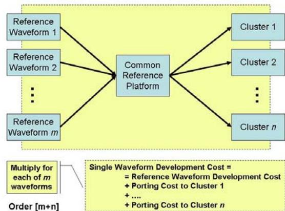
Figure 3. Waveform porting costs with a Common Reference Platform. Costs can be reduced to order of  $[m + n]$ .
