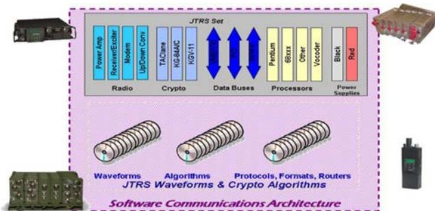
Figure 1. Joint Tactical Radio System software defined radio. (Figure: JTRS Public Distribution)
