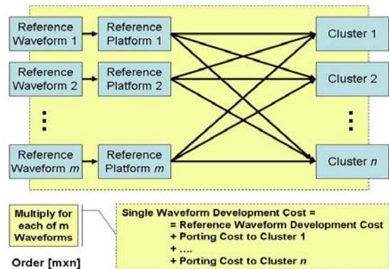
Figure 2. Waveform “porting” costs without a Common Reference Platform can grow by order  $[m \times n]$ .
