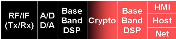
Figure 4. An example of a Red/Black isolated radio platform, in which the protected “Red” side is isolated from the “Black” side by a cryptographic boundary.
