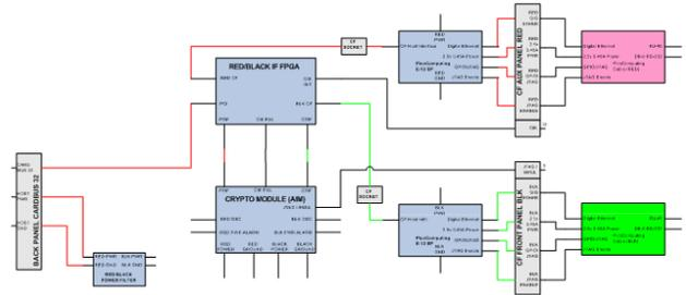
Figure 7. Common interfaces to cryptographic modules (CICM) APIs are employed on this concept for a Cryptographic Development Module for the SCA Common Reference Platform. The version employing the Advanced INFOSEC Machine (AIM) is shown in this figure.
