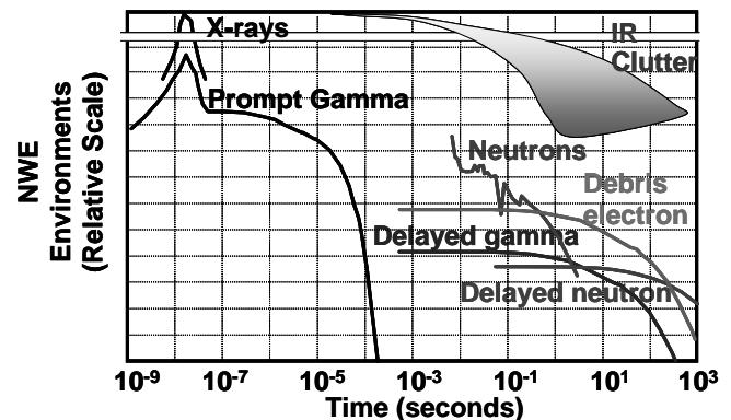
**Figure 2.** Nuclear Weapon Radiation Environment vs. Time
