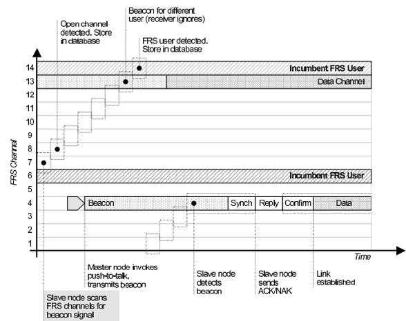
Fig. 2. Example of spectrum access behavior of the CIREN system
