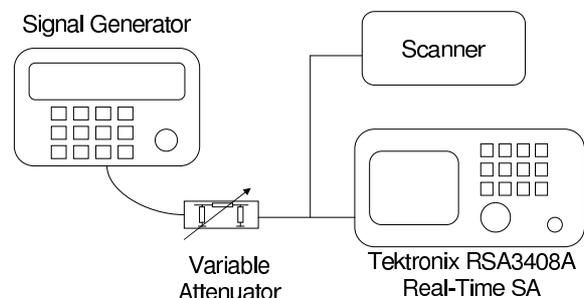
Fig. 3. Sensitivity test setup
