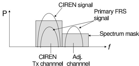
Fig. 6. Signal location for vacancy time measurement
