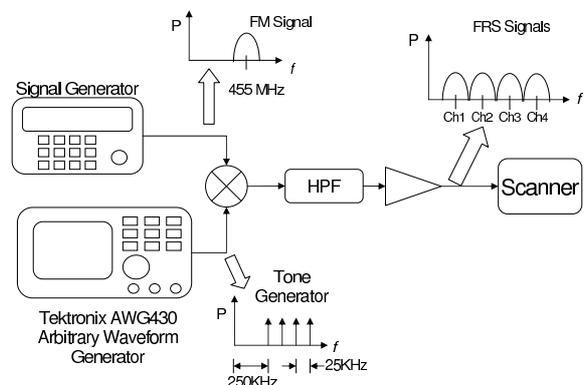
Fig. 4. Occupied channels test setup
