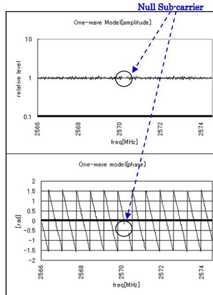
Figure 5 Amplitude and Phase Spectrum Characteristics at the Monitoring Point in the case of Non-fading.
