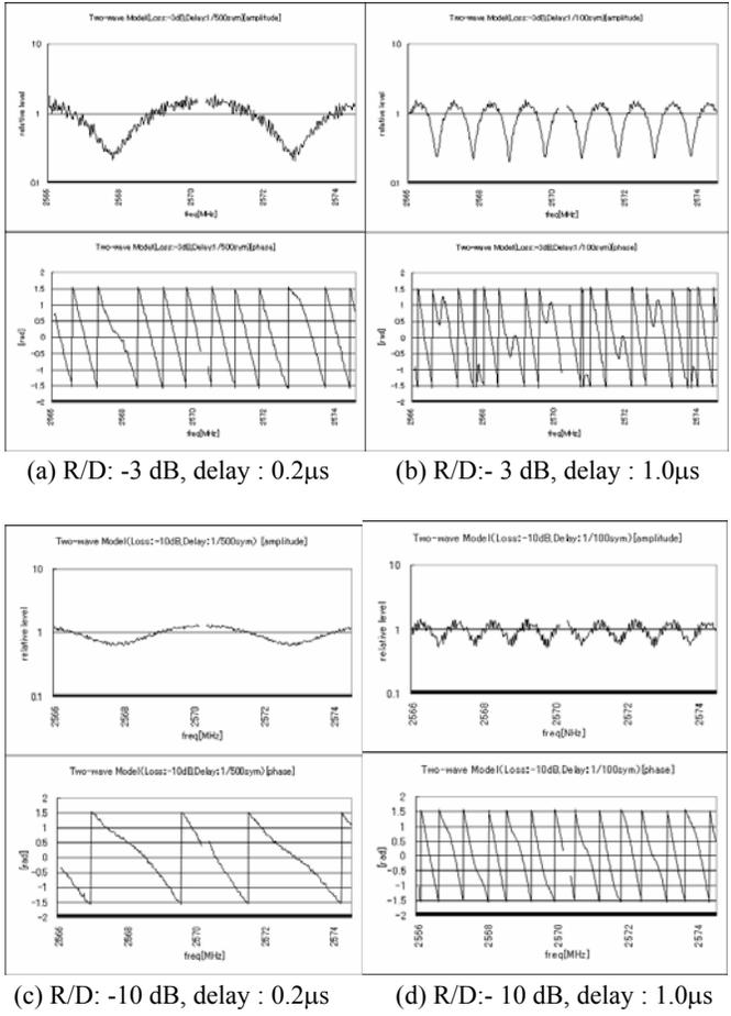
Figure 6 Monitoring Results in Two-path model
