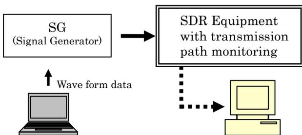
Figure 4 Experimental Configuration for Evaluation of Transmission Channel Monitoring Function.
