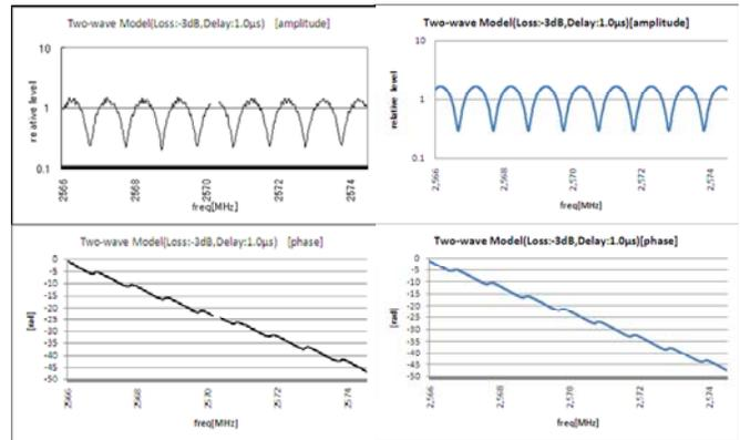
(a) Experimental Transfer Function (equivalent to Fig.6 (b)) (b) Analytical Transfer Function (equivalent to Fig.6 (b))
