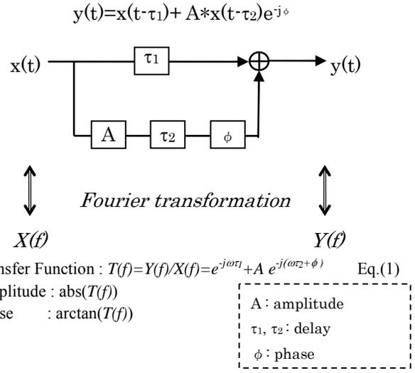
Figure 7 Channel model and Transfer Function
