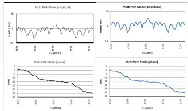
(a) Experimental Transfer Function (b) Analytical Transfer Function
