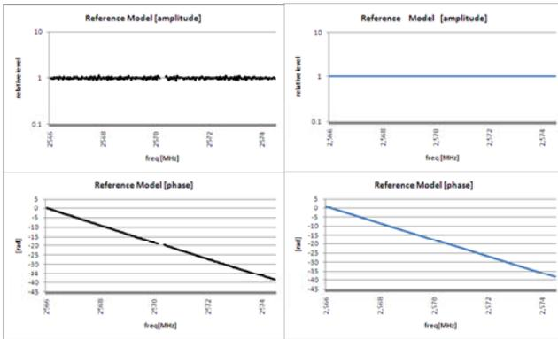
(a) Experimental Transfer Function (equivalent to Fig. 5) (b) Analytical Transfer Function (equivalent to Fig. 5)
