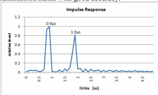
Figure 10 Impulse Response calculated from Fig. 6 (b) (R/D:- 3dB, delay : 1.0 $\mu$ s).
