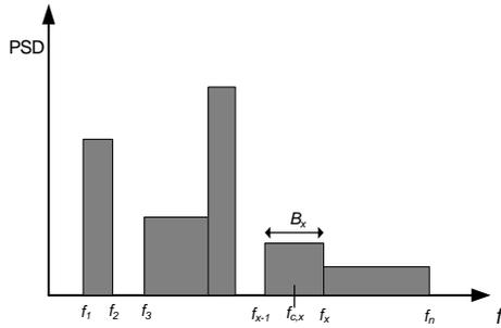
Figure 2. PSD of N spectrum sub-bands.
