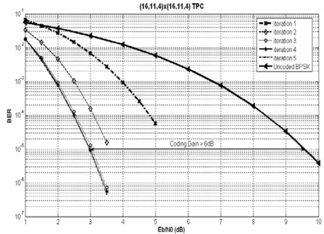
Fig. 3. BER vs.  $E_b/N_0$  of product code [BCH (16,11,4)<sup>2</sup>] on a Gaussian Channel
