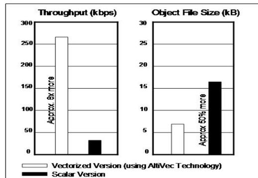
Fig. 4. TPC: Vector vs. Scalar Implementation Results (Both Implementations were carried out on MPC7447A@1.0 GHz)
