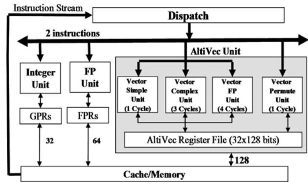
Fig.2. AltiVec architectural diagram with three Vector ALUs and one Permute unit
