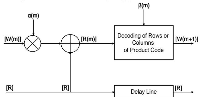
Fig.1. Block diagram of elementary TPC decoder ( $m^{\text{th}}$  half-iteration)
