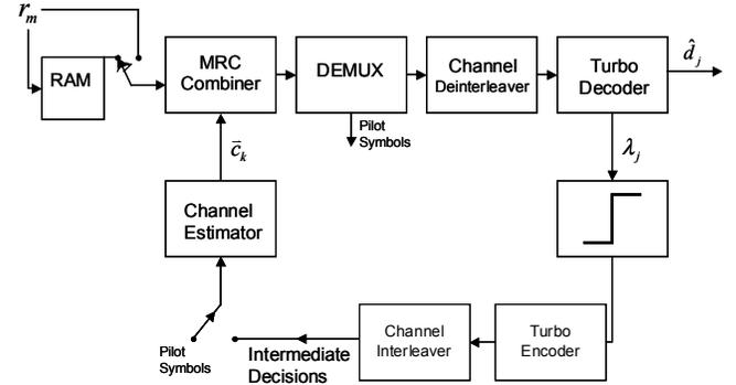
Figure 2 Turbo-Aided Receiver Model
