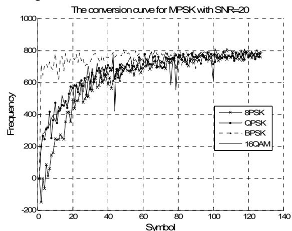
Figure 5: The frequency tracking curves for MPSK
