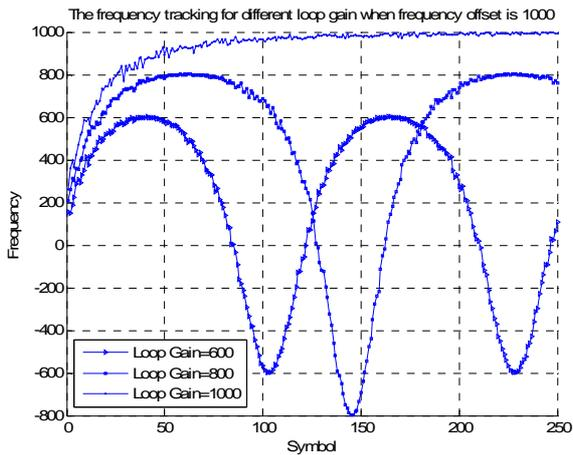
Figure 6: The relationship between loop gain and maximum value of frequency offset
