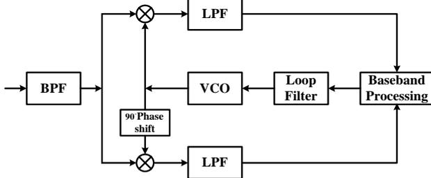
Figure 2. Block diagram of baseband carrier recovery
