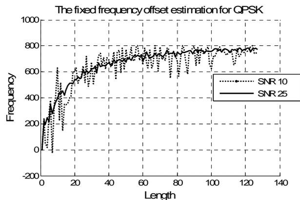
Figure 4: The frequency tracking curve for QPSK
