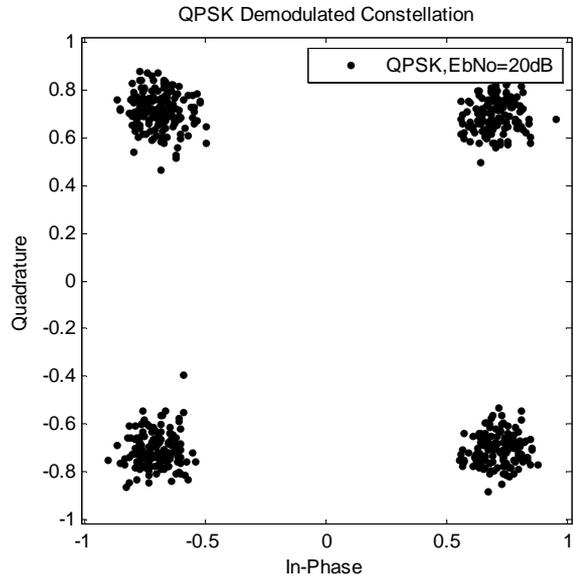
Figure 8 QPSK Demodulated Constellation
