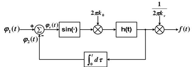
Figure 1: The phase-locked loop architecture
