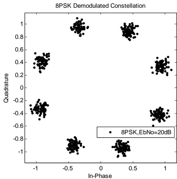
Figure 9 8PSK Demodulated Constellation
