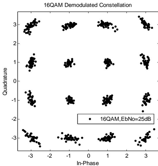
Figure 10 16QAM Demodulated Constellation
