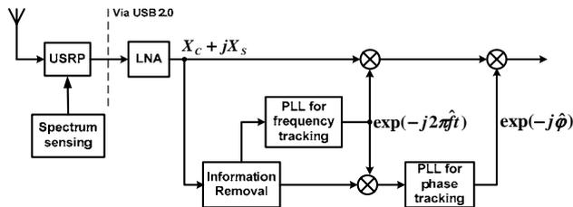
Figure 3: Universal synchronization system frame
