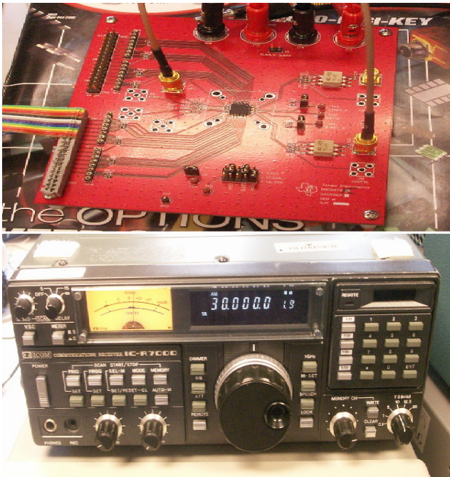
Figure 6 Hardware of the DAC and Radio Scanner
