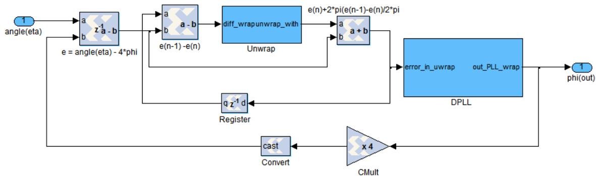
Fig. 6. The EPLL in system generator for DSP
