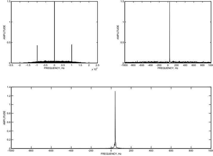
Fig. 4. The power spectrum of  $y^4[n]$  (a) before filtering, (b) after low pass filtering and decimation, (c) after the line enhancer
