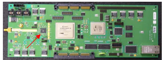
Figure 1. Layout of the EVB101-RX and EVB101-TX. A red arrow indicates the location of the Lycon™ chips.
