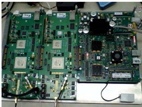
Figure 3. Photograph of the WMB101 WiMax Evaluation Platform. The platform consists of three boards (from left to right): the EVB101-TX, the EVB101-RX and the HDP102 by picoChip.
