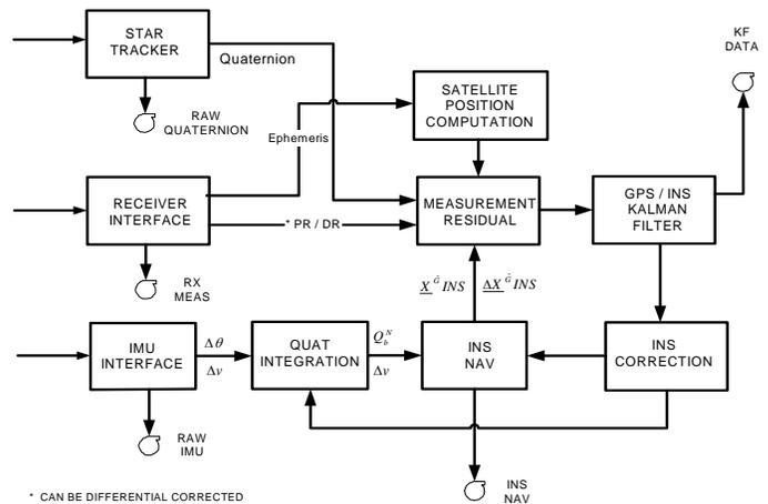
Figure 7 NAVSYS GPS/Inertial Filter Software
