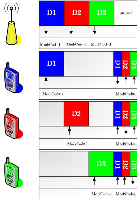
**Figure 4. Downlink cooperative scenario using the principle of OFDM and FDMA**
