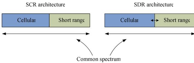
**Figure 3. Spectrum allocations using an SCR implementation and an SDR implementation**
