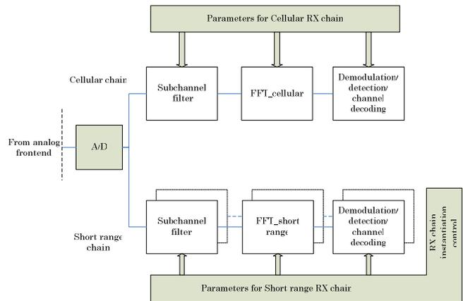
Figure 7 SDR receiver concept
