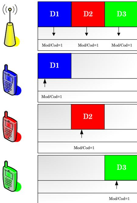
**Figure 5 Carrier allocation scenario with no cooperation and static carrier assignment**
