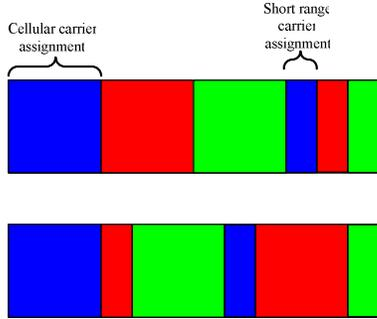
**Figure 6 Example of non-contiguous carrier assignment**
