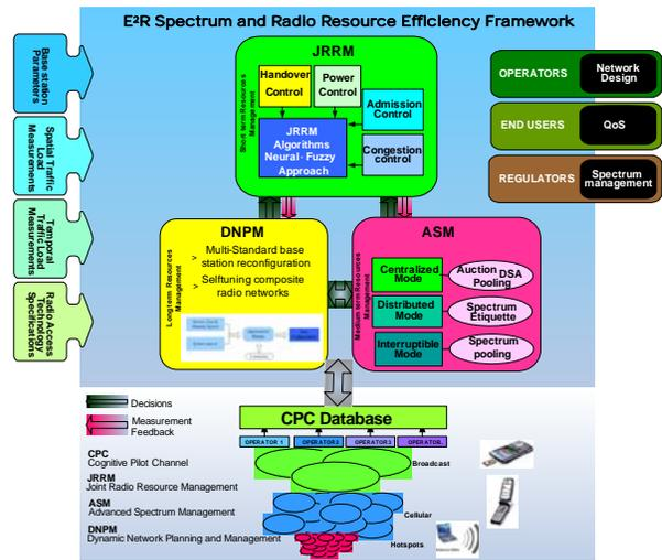
Fig. 4: E<sup>2</sup>R II Spectrum and Radio Resource Efficiency Framework
