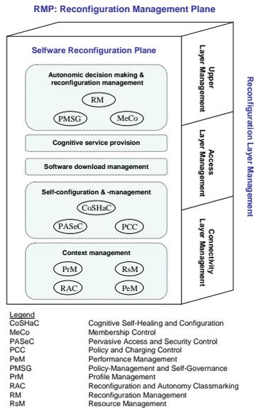
Fig. 3: The Reconfiguration Management Plane Model for Autonomously Reconfigurable Elements.
