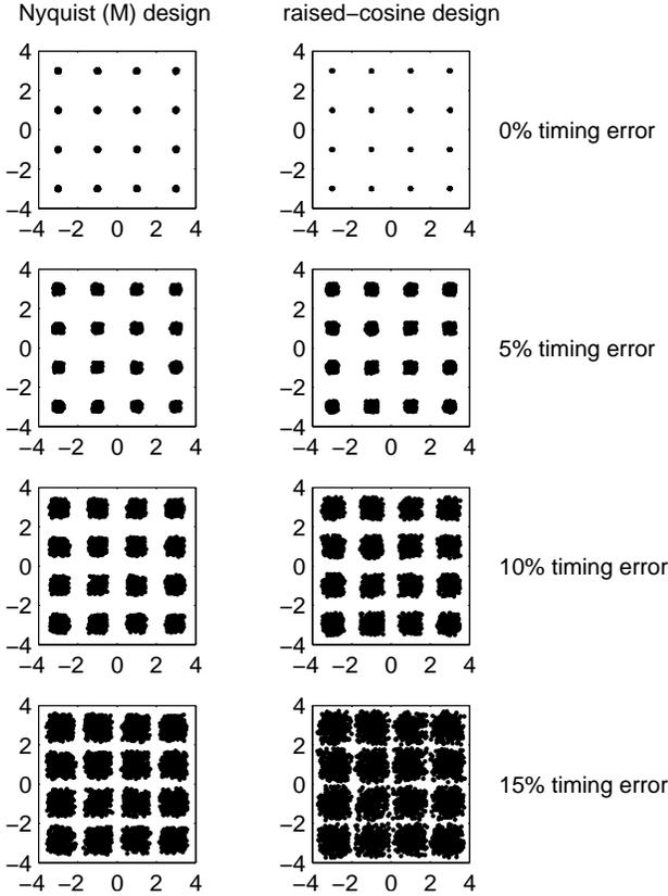
Fig. 3. Demonstration of the robust behavior of a Nyquist (M) filter to timing phase offset, through eye patterns. The eye patterns arising from a raised-cosine pulse are also presented.
