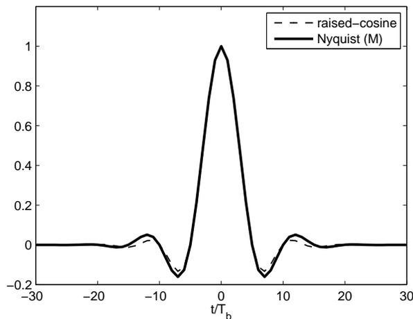
Fig. 2. Combined response of a pair of matched square-root raised-cosine and square-root Nyquist ( $M$ ) filters.
