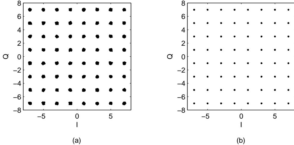
Fig. 1. Symbol constellation/eye pattern of a 64-QAM symbol sequence after passing through a pair of matched filters. (a) square-root raised-cosine filter. (b) square-root Nyquist ( $M$ ) filter.
