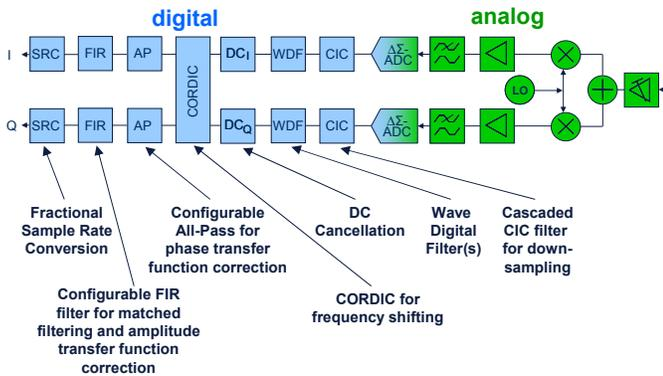
Fig. 3. Proposed E<sup>2</sup>R RF IC receiver architecture.
