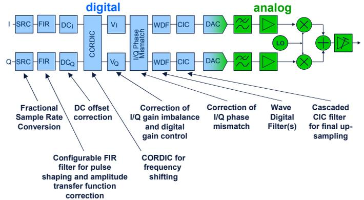
Fig. 4. Proposed E<sup>2</sup>R RF IC transmitter architecture.
