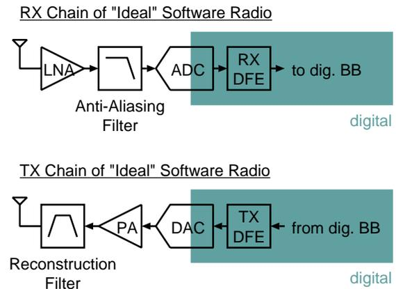
Fig. 2. *Ideal* SDR receive (a) and transmit (b) paths.
