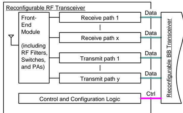
Fig. 1. RF transceiver with  $x$  concurrent receive and  $y$  concurrent transmit paths.
