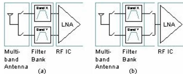
Fig. 5. A possible realization of a multi-standard (GSM900, WCDMA, and 2.4 GHz WLAN) and possible interfaces to the RF IC (a), (b).
